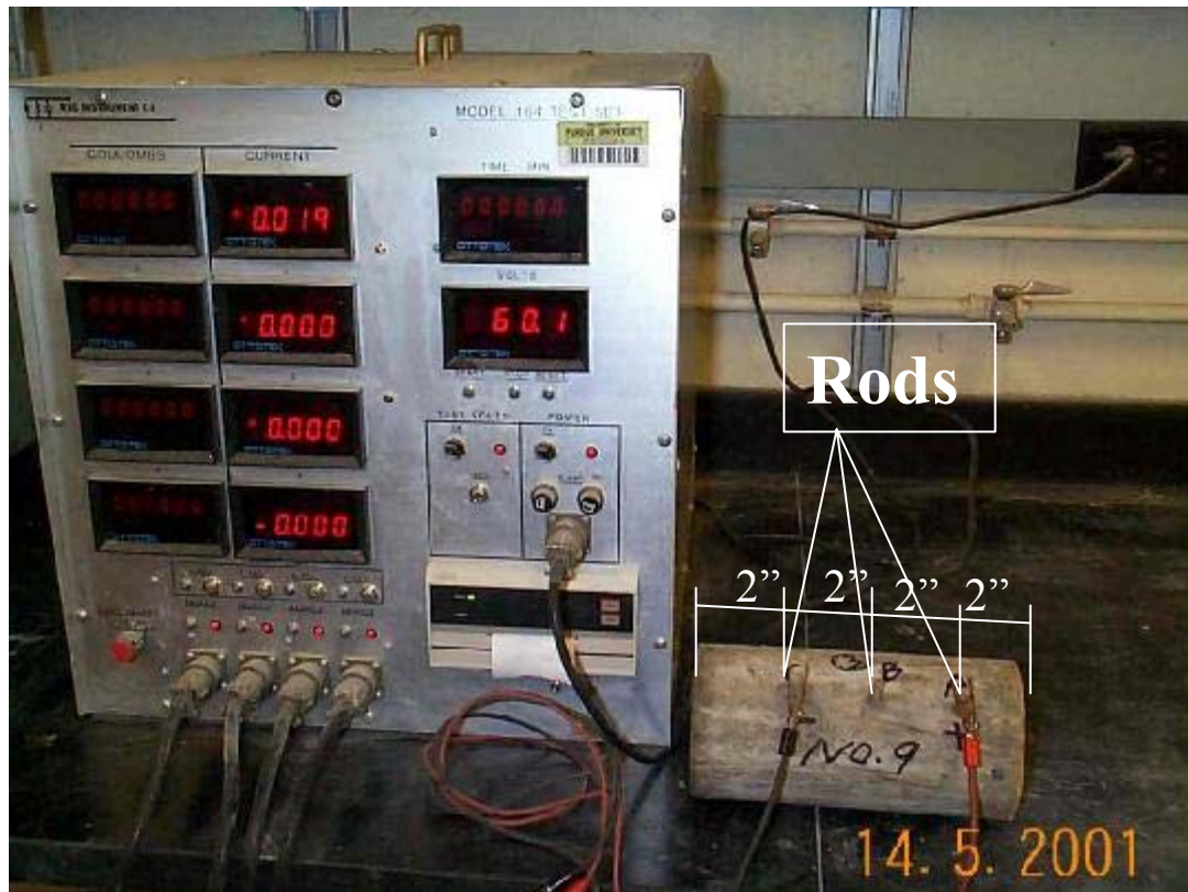
Figure 5.27: Set-up of DC Electrical Resistance Test
