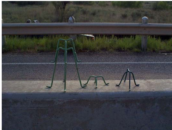
Figure 5.1: Epoxy Coated Steel Chairs (Sierrita de la Cruz Creek Bridge, Amarillo, Texas, 2000)
