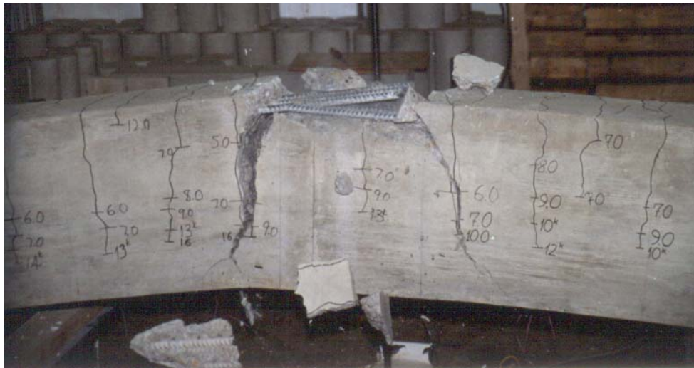
(b.) Failure of B-S-2
