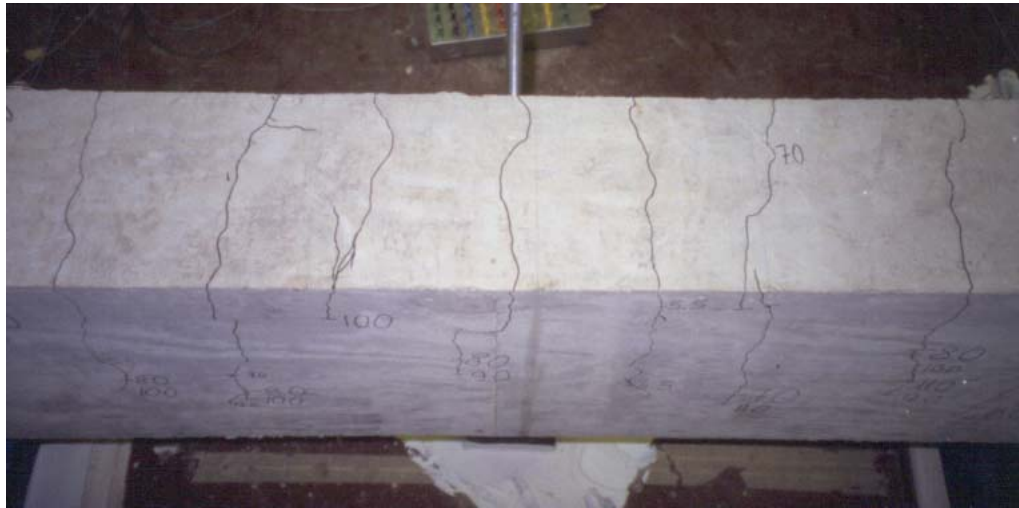
(a.) Top View of Specimen B-S-1 at 40 ksi
