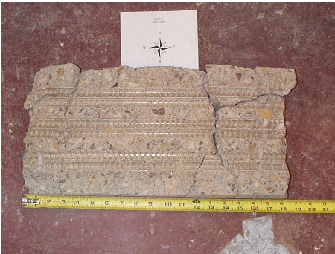
Figure 3.9: Splitting Failure Modes
