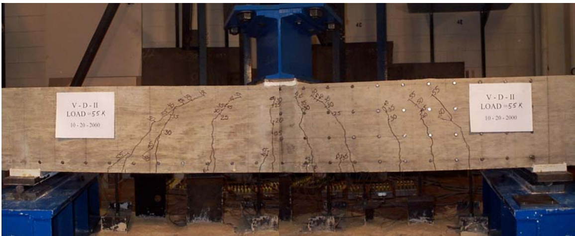
Figure 4.9: Specimen V-D-2 Prior to Failure
