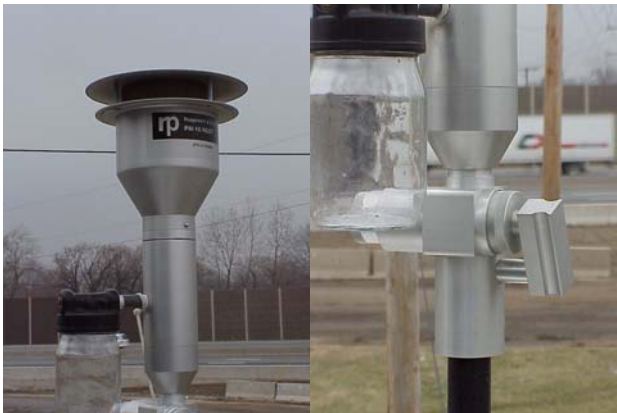
Figure 2.5 : Size Selective Inlets: PM 10 Impactor on left, Sharp Cut Cyclone on right.
