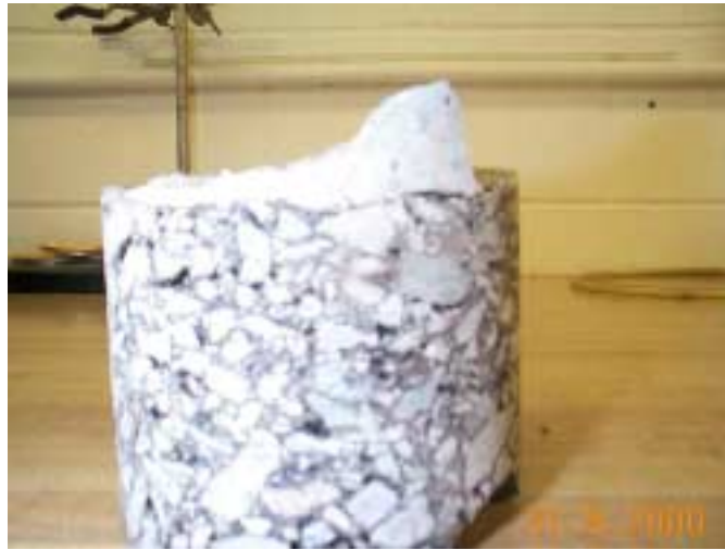
Figure 5.17 Failure of UTW core at the concrete section
