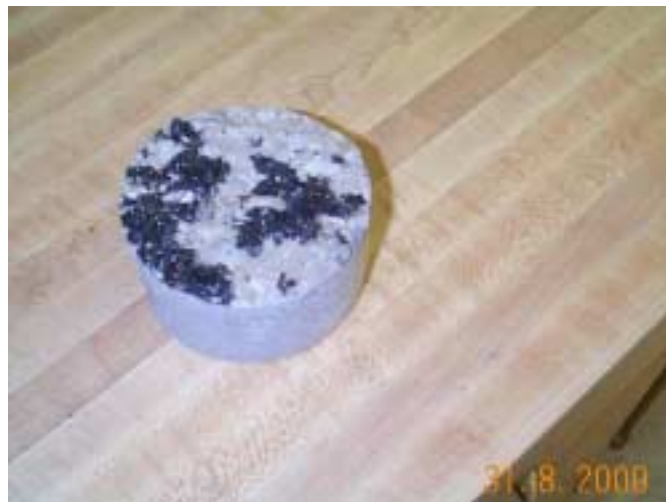
Figure 5.18 Failure of UTW core at the interface along with asphalt stuck to the surface
