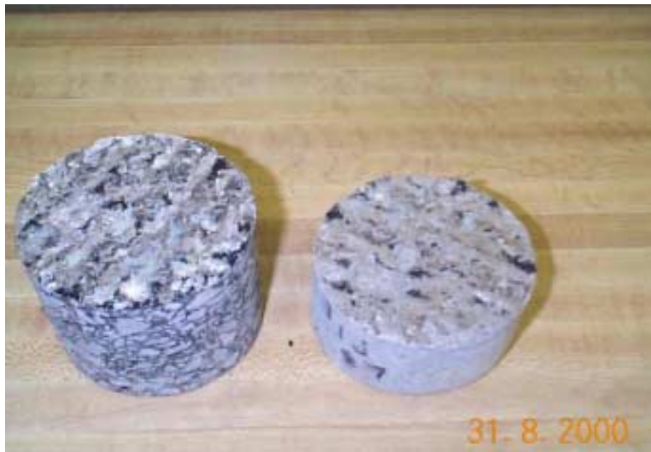
Figure 5.16 Typical failure of a UTW specimen in the Iowa shear test
