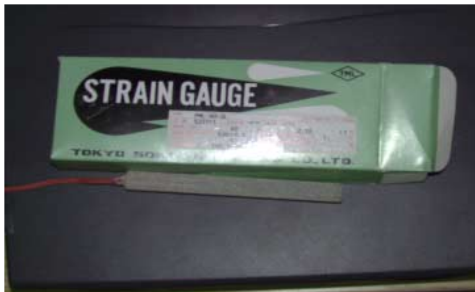
Figure 3.4 Concrete embedment gages (PML-60-2L) used in UTW
