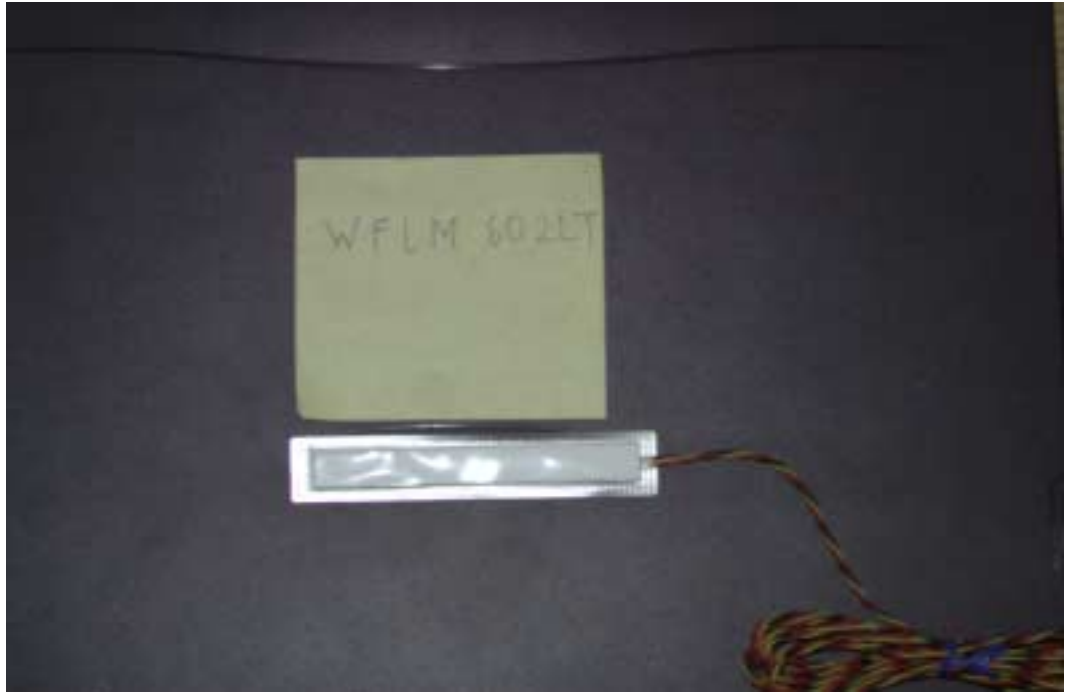
Figure 3.3 Non-encapsulated gage (WFLM-60-2LT) used on the asphalt surface
