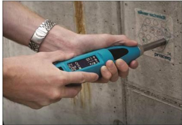
Figure 2.1 RH Test Performing on a Concrete Surface.
