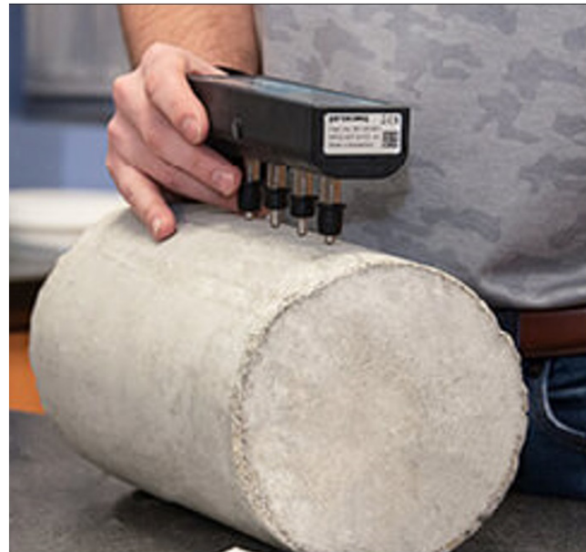
Figure 2.8 Surface ER Test Being Performed on a Concrete Cylinder Using a Wenner Four-Probe Device.
