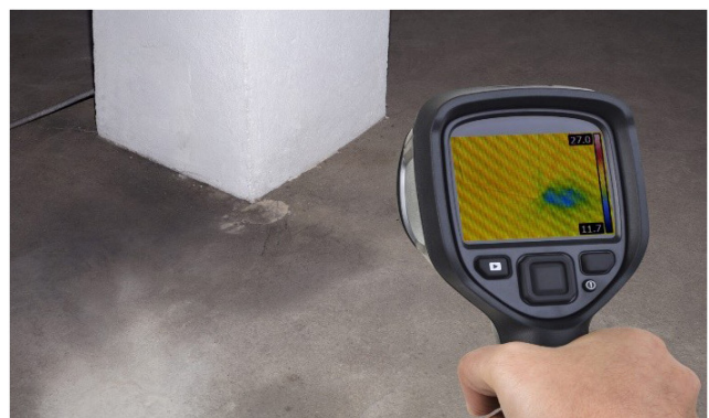
Figure 2.7 IRT Being Used to Detect Thermal Anomalies in a Concrete Structure.
