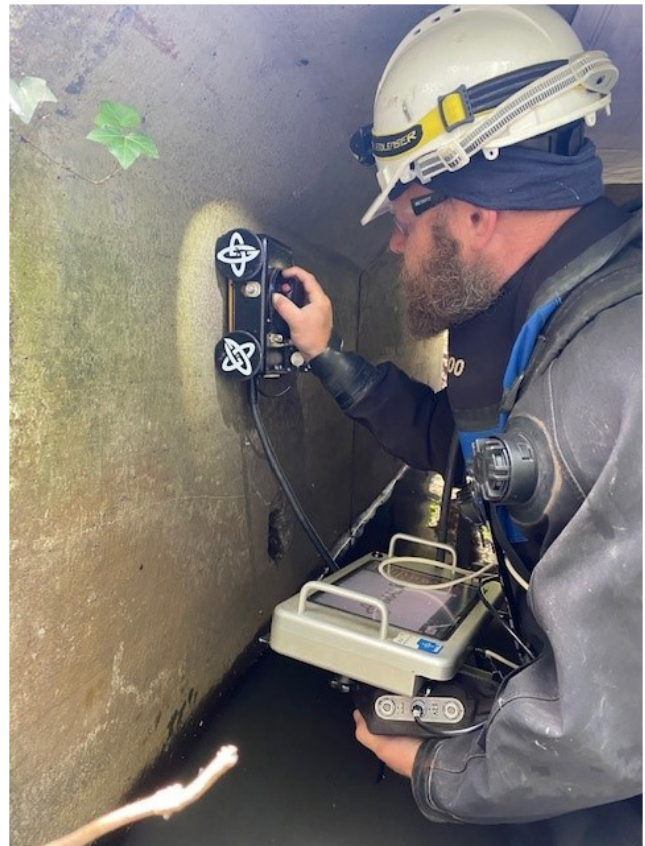
Figure 2.5 GPR Testing on a Vertical Concrete Member.
