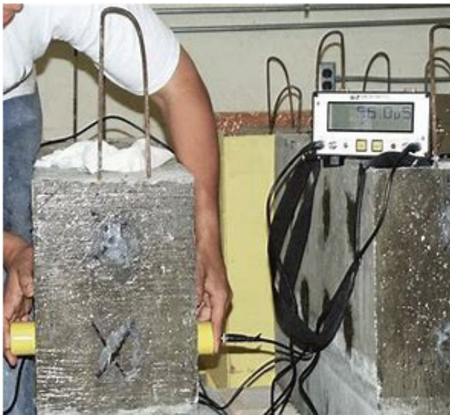
Figure 2.2 Two-Sided UPV Test on Concrete for Internal Quality Assessment.
