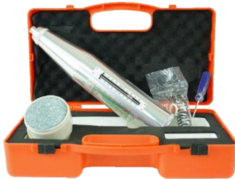
Figure 28 Controls, Concrete Test Hammer
