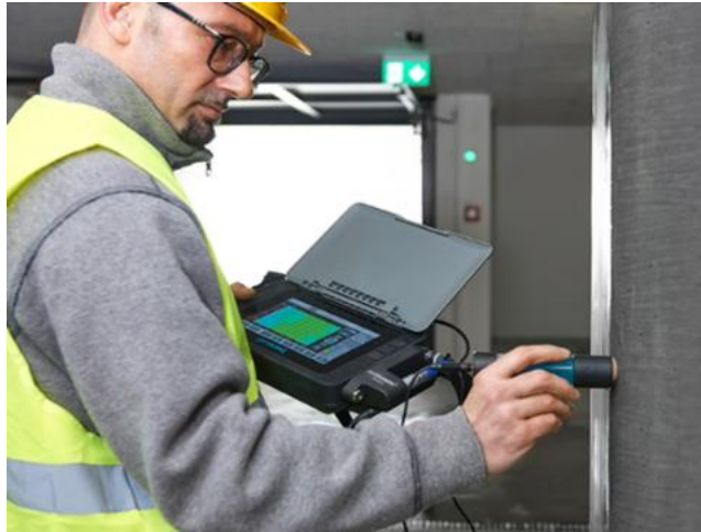
Figure 53 Proceq, Profometer Corrosion
