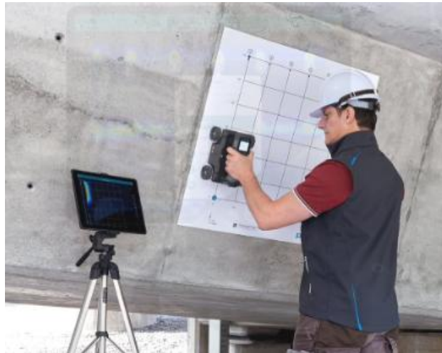
Figure 1 Grid paper for GPR mapping and data collection
