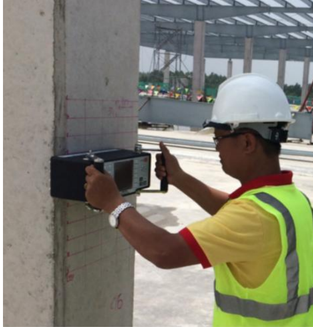
Figure 18 Acoustic Control Systems, A1040 MIRA
