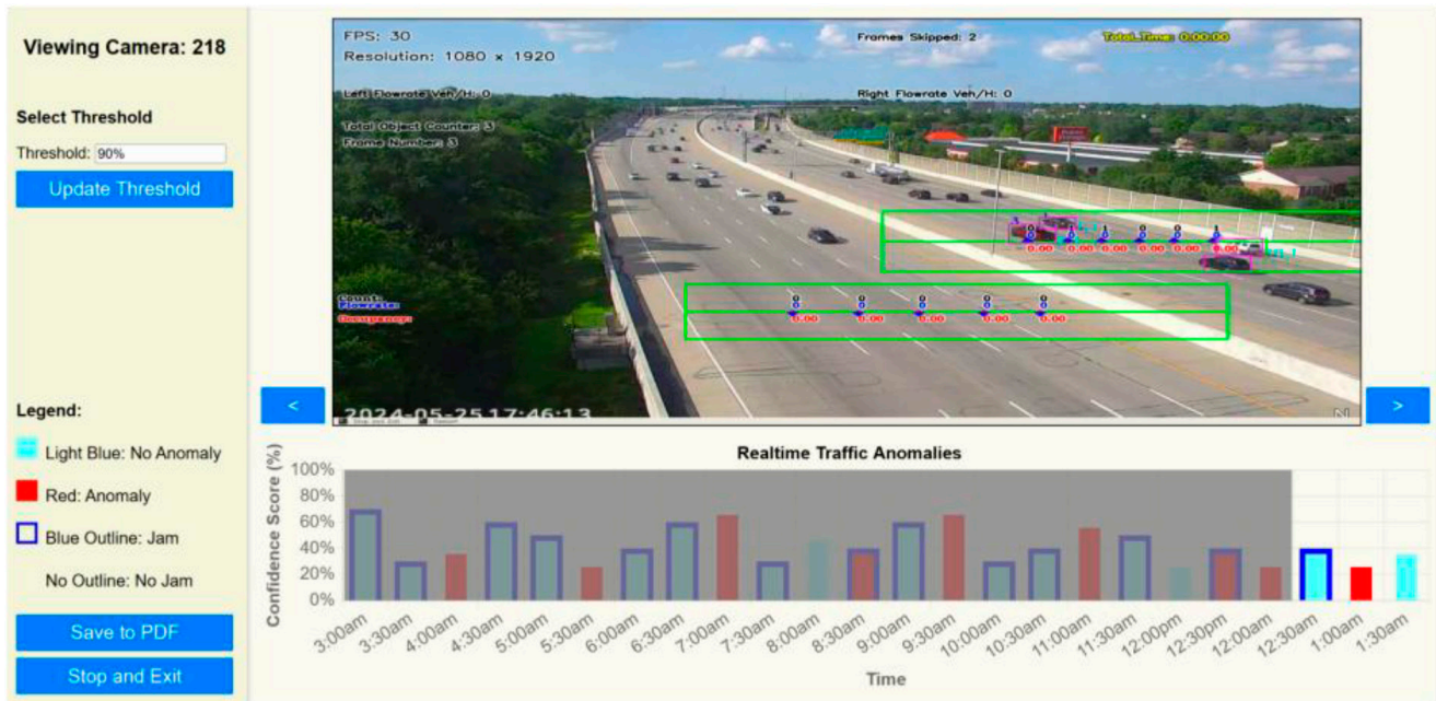
Figure 3.16 (b) Real-Time User Interface for Viewing Anomaly Detection Results as They Are Processed From the Live Camera Feed.
