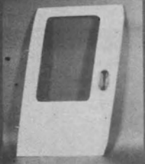
LITTER DOOR KEVLAR/EPOXY FABRIC TWO SKINS - HOLLOW SECTION MASS (kg) 3.72 SIZE (m) 1.17 x 0.66
