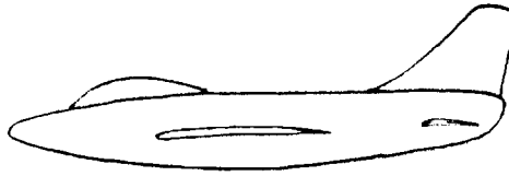
Contiguous Skin Model of the Aircraft for Diffusion Calculations
