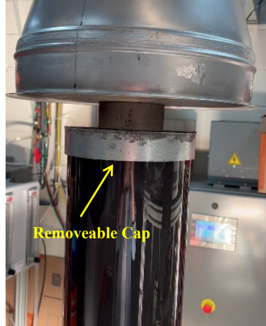
Figure 5. Removeable cap used in OSB experiments to minimize air entrainment at top of quartz tube
