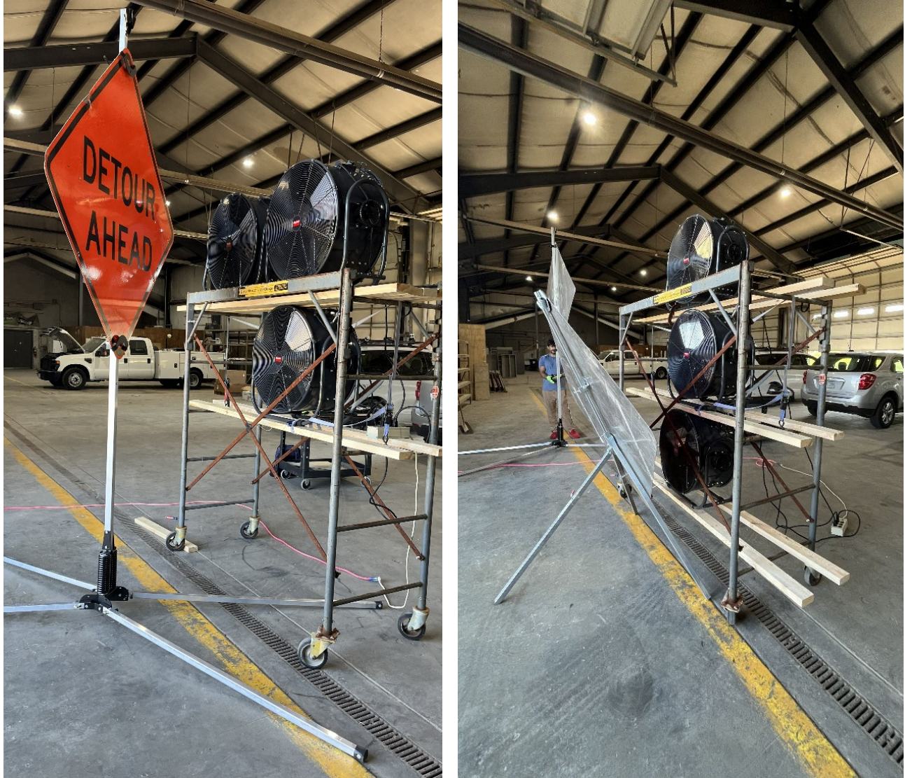
Figure 7. Photos. Experimental setup using fans to generate artificial winds: (left) tall four-legged sign support system with springs, and (right) tripod sign support system.
