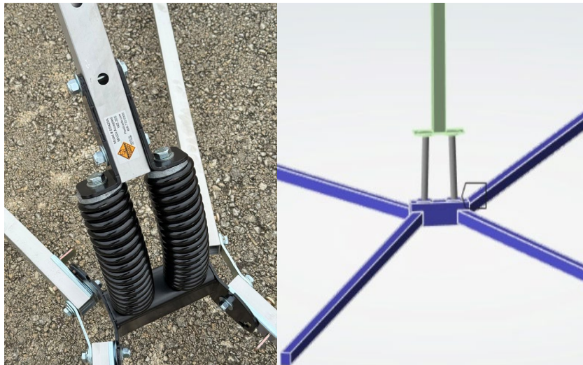
Figure 14. Photo and Illustration. Equivalent structural idealization of spring assemblies for finite-element modeling: (left) photo from field experiment; (right) model in ANSYS Mechanical 2025.
