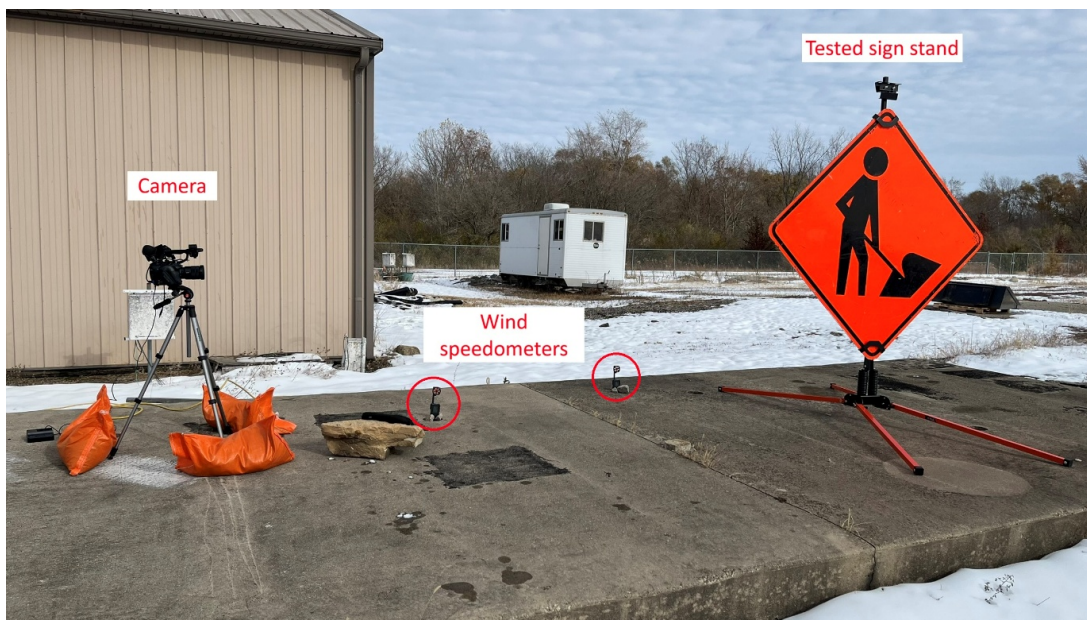
Figure 9. Photo. Experimental setup to measure the profile of the wind causing deflections to a spring-based sign support system.
