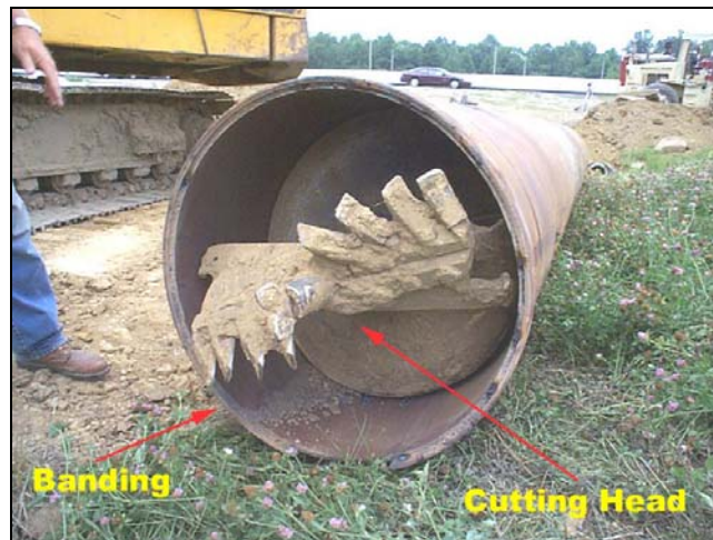
Figure 2.6 Cutting head and partial banding
