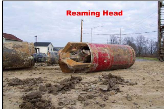
Figure 2.38 Reamer for PTMT
