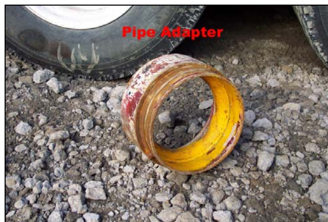
Figure 2.42 Pipe adapter for PTMT
