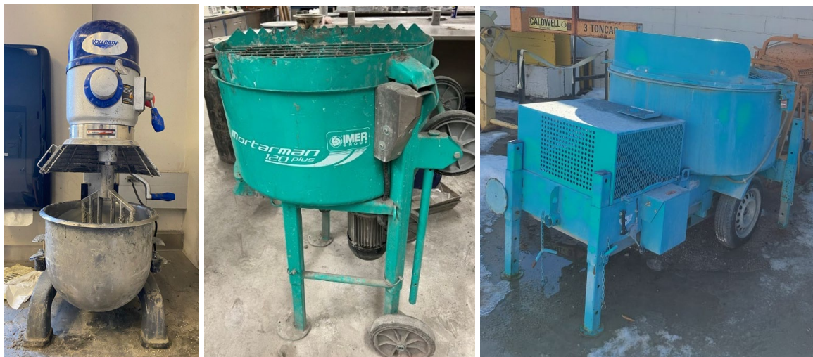
Figure 3.1 Mixers used in UHPC batching (left to right: Vollrath benchtop mixer, IMER 120 mixer, and IMER 750 mixer)
