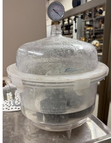
(b) Sample preparation in vacuum saturation chamber
