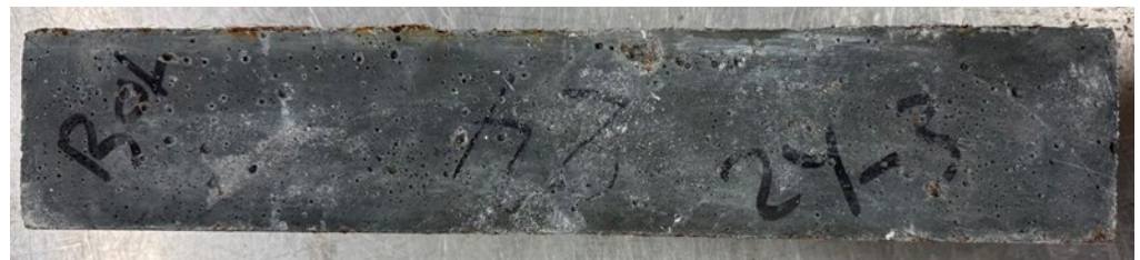
Figure 6.21 Representative specimens after 300 cycles of freezing-thawing test.
