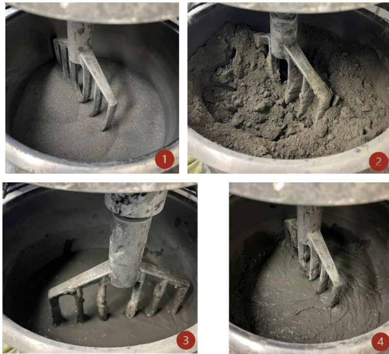
Figure 3.2 Appearance of the mixtures at various stages of the mixing process
