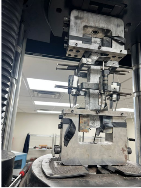
Figure 3.12 Uniaxial tensile strength test setup.
