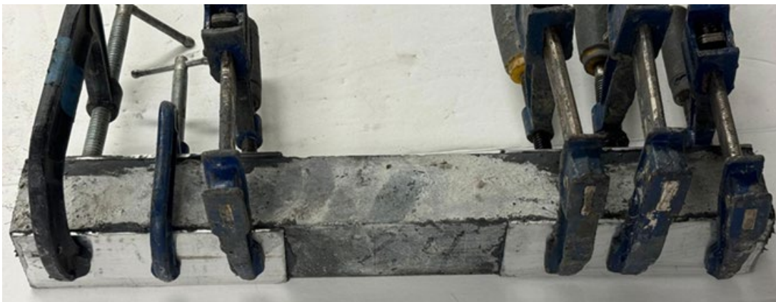
Figure 3.13 Clamping of Specimens.
