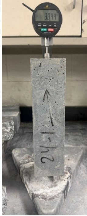
Figure 3.21 Drying shrinkage test setup.
