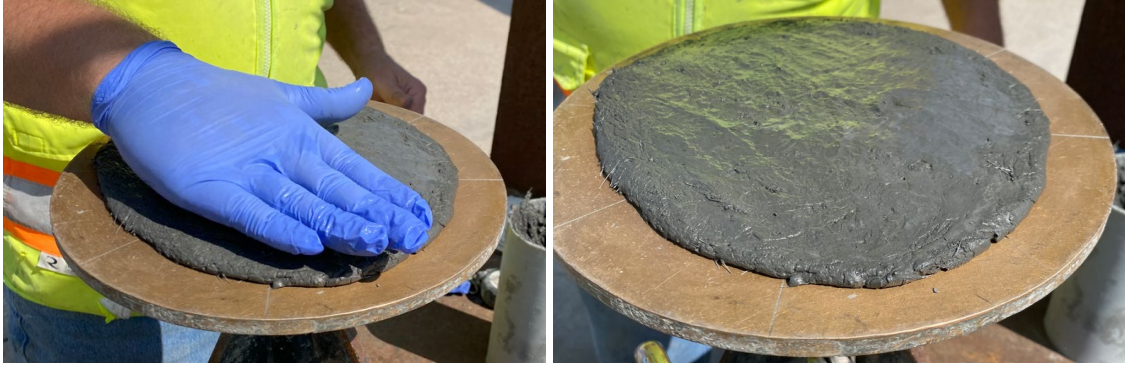
Figure C.6 Material reacts well under external energy (vibration).
