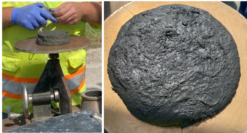
Figure C.5 Flow after adjustment (4.25" static, 7.5" dynamic).
