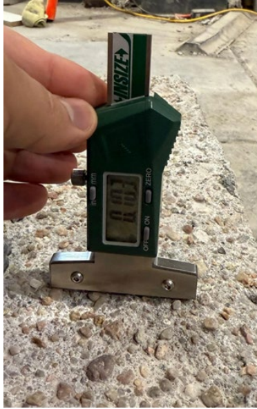
Figure 6.7 Measuring surface roughness using a caliper.
