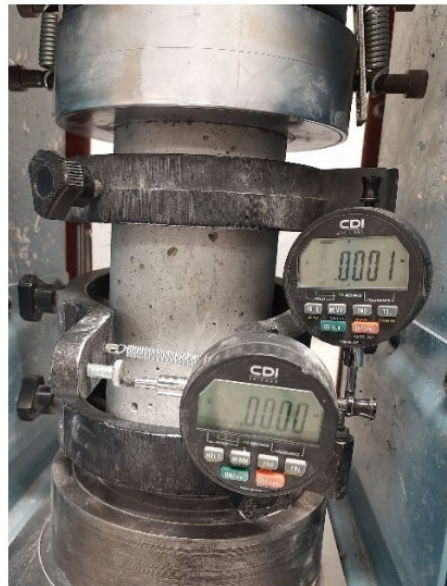
Figure 3.8 Static modulus of elasticity test setup.
