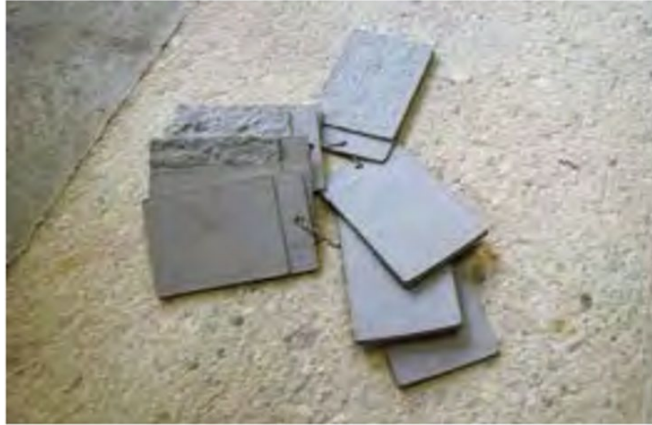
Figure 2.2 CSP Comparator Chips (ICRI 310.2R 2013).
