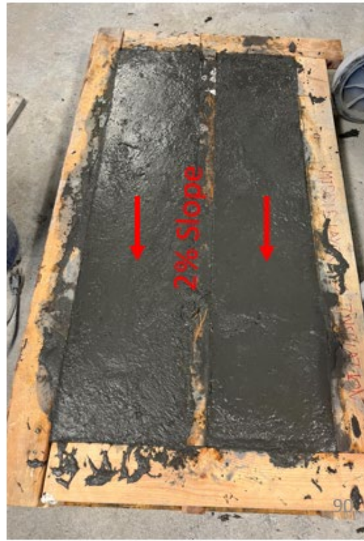
Figure 4.18 Casting the small-scale slabs with UHPC overlay.
