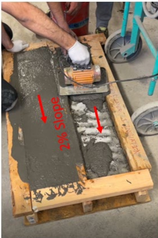
Figure 4.18 Casting the small-scale slabs with UHPC overlay.
