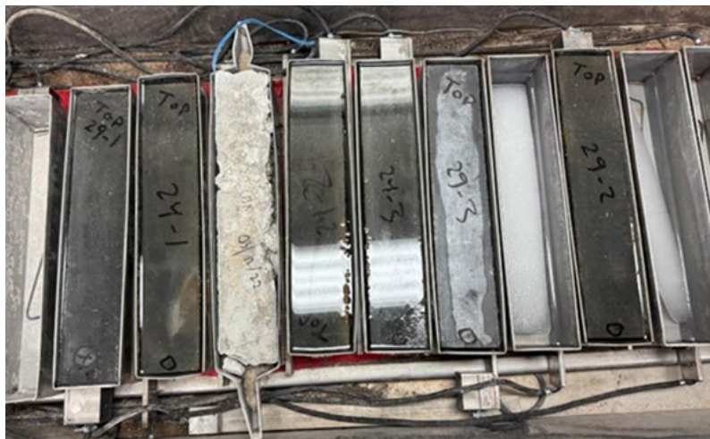
Figure 3.17 UHPC specimens in the freeze-thaw chamber.
