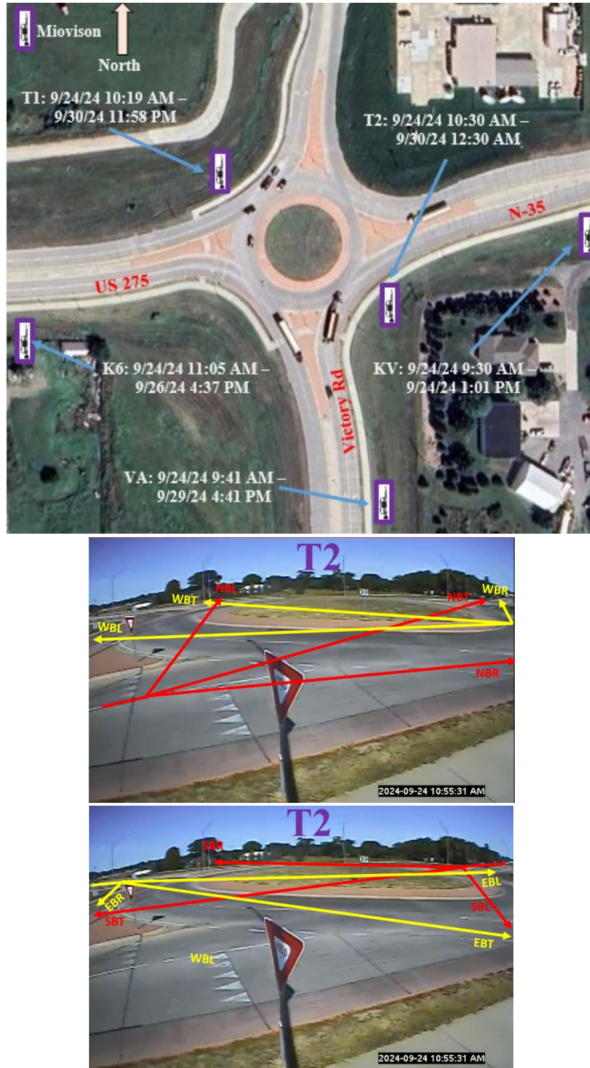
Figure A.8 Data collection device locations and corresponding traffic movements at the Norfolk site
