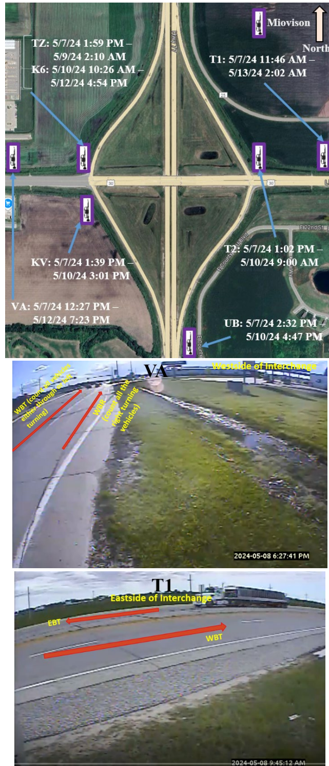
Figure A.10 Data collection device locations and corresponding traffic movements at the Fremont site
