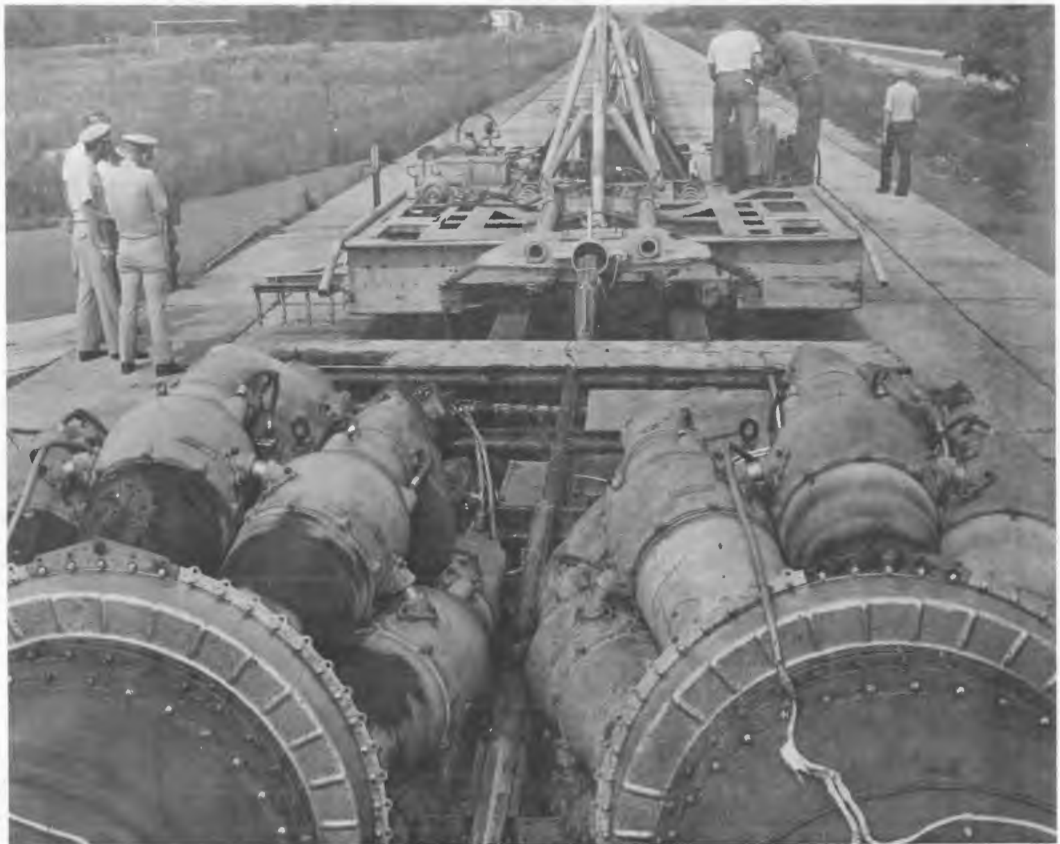
FIGURE 1. JET-POWERED PUSHER CAR FOR PROVIDING PRESELECTED SPEEDS TO TEST EQUIPMENT
