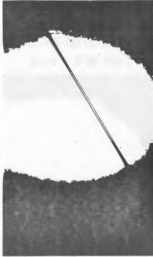
JET-A + 0.3% AM-1 NOZZLE FLOW DOWNWARDS NO FREESTREAM VELOCITY JET EXIT VELOCITY 3.2 m/sec JET EXIT DIA 0.88 mm
