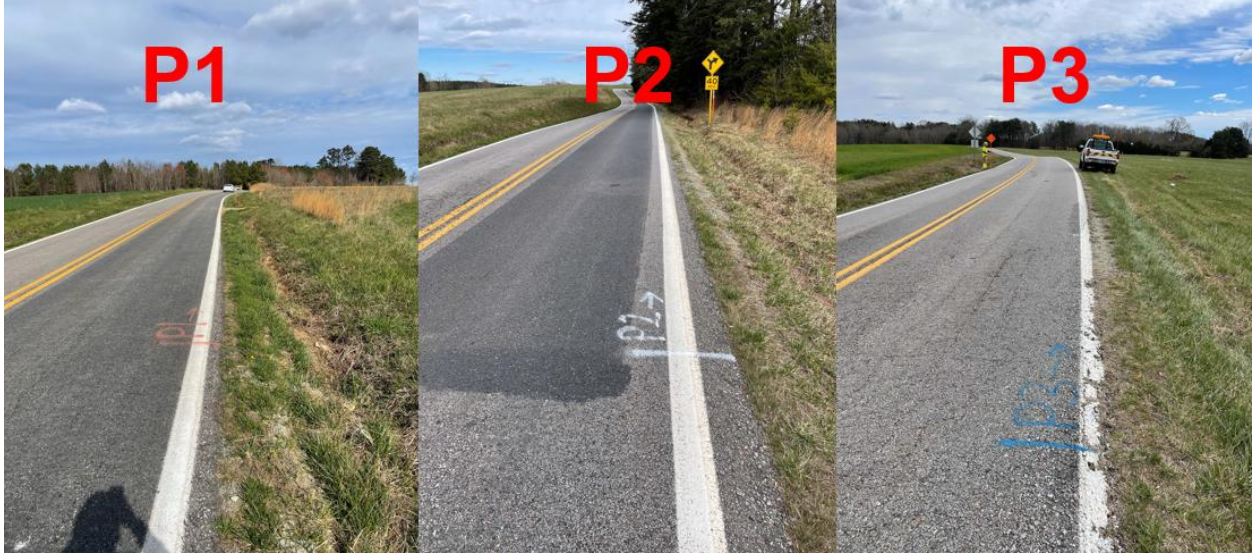
Figure 21. Images of Surface Appearance Approximately 6 Months after Spray-on Rejuvenator Application for Route 750. Treated lane is shown on the left, and untreated lane is shown on the right. P1–P3 denote segments receiving spray-on rejuvenator application.
