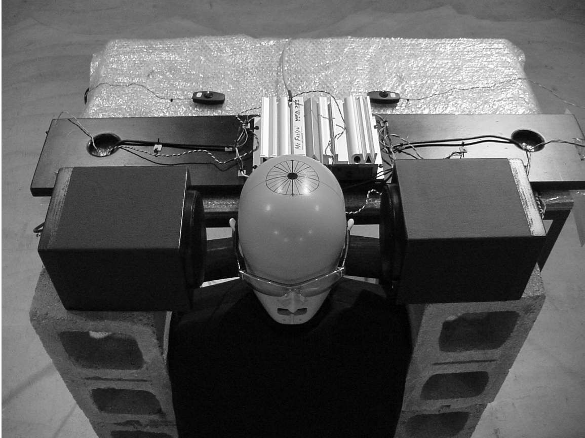
Figure 5.7: Photo of the TechnoFirst Prototype External ANC System and the head and torso simulator.
