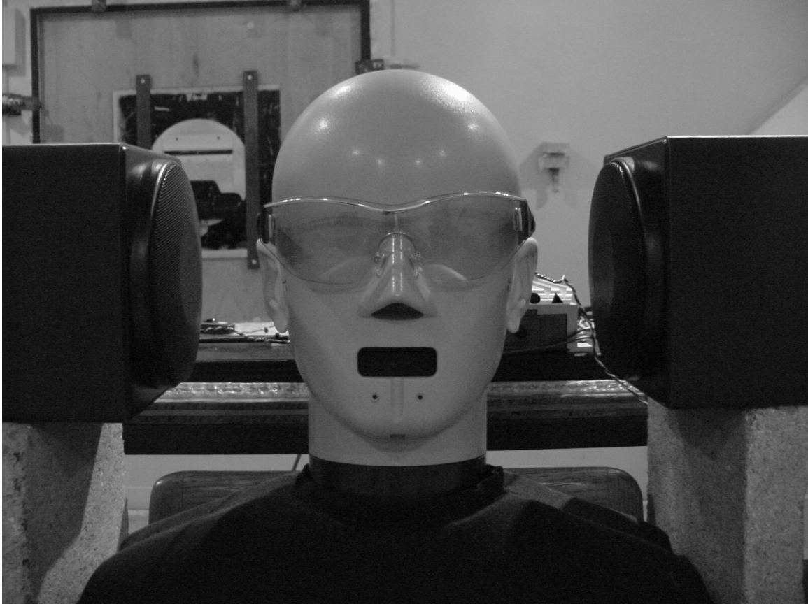
Figure 5.2: Location of the TechnoFirst ANC system with respect to the head and torso simulator.
