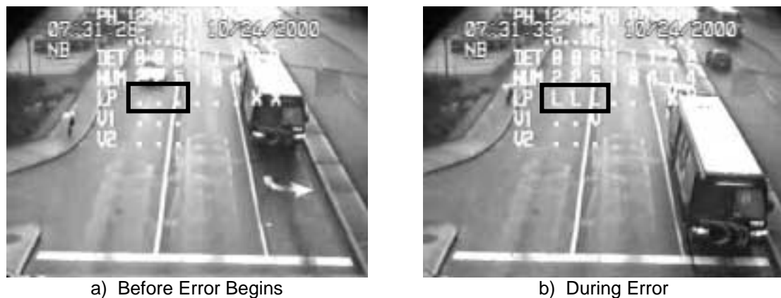
Figure 4-5: Example Screen Captures of L1V0 Error Caused by Inductive Loops (Before Recalibration, System 1)
