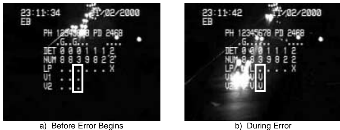
Figure 4-2: Example Screen Capture of L0V1 Discrepancy Caused by Headlight Glare in Left Turn Lane (Systems 1 & 2, Before Recalibration)
