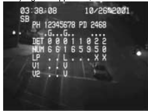
d) Vehicle with no lights successfully detected by loops and both video detectors (Detector 01)
