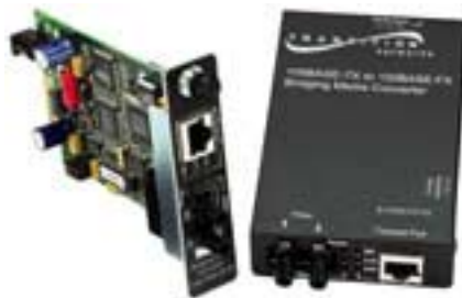
Figure 3-13: 100 Base-T to 100 Base-FX Media Conversion (NW04, CIVL02)
