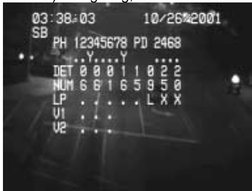
c) Lighted approach, vehicle with no lights approaching back loop (Detector 9)
