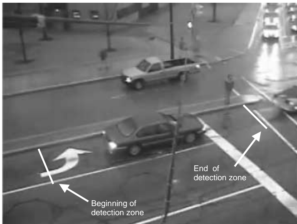
Figure 7-4: Screen Capture of Northbound Left Turn Lane During a Ground Truth Data Collection
