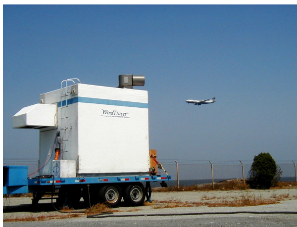
Figure 8. B-747 aircraft above the optical pulsed lidar. The WindTracer ® Lidar is manufactured by CLR Photonics.
