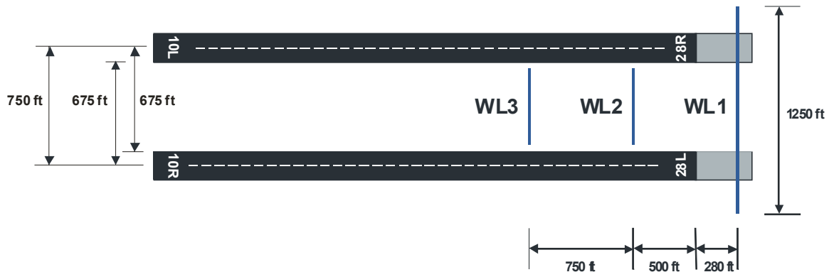
Figure 4. Relevant dimensions between Runways 28L and 28R as well as positions of the three windlines relative to the runways.
