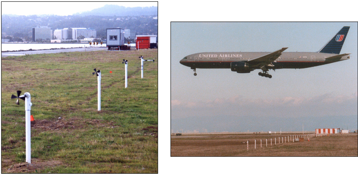
Figure 7. (Left) Close-up view of windline 1 showing the 3-foot high poles and the propeller anemometer on top of each pole. (Right) B-777 aircraft landing over windline 1.
