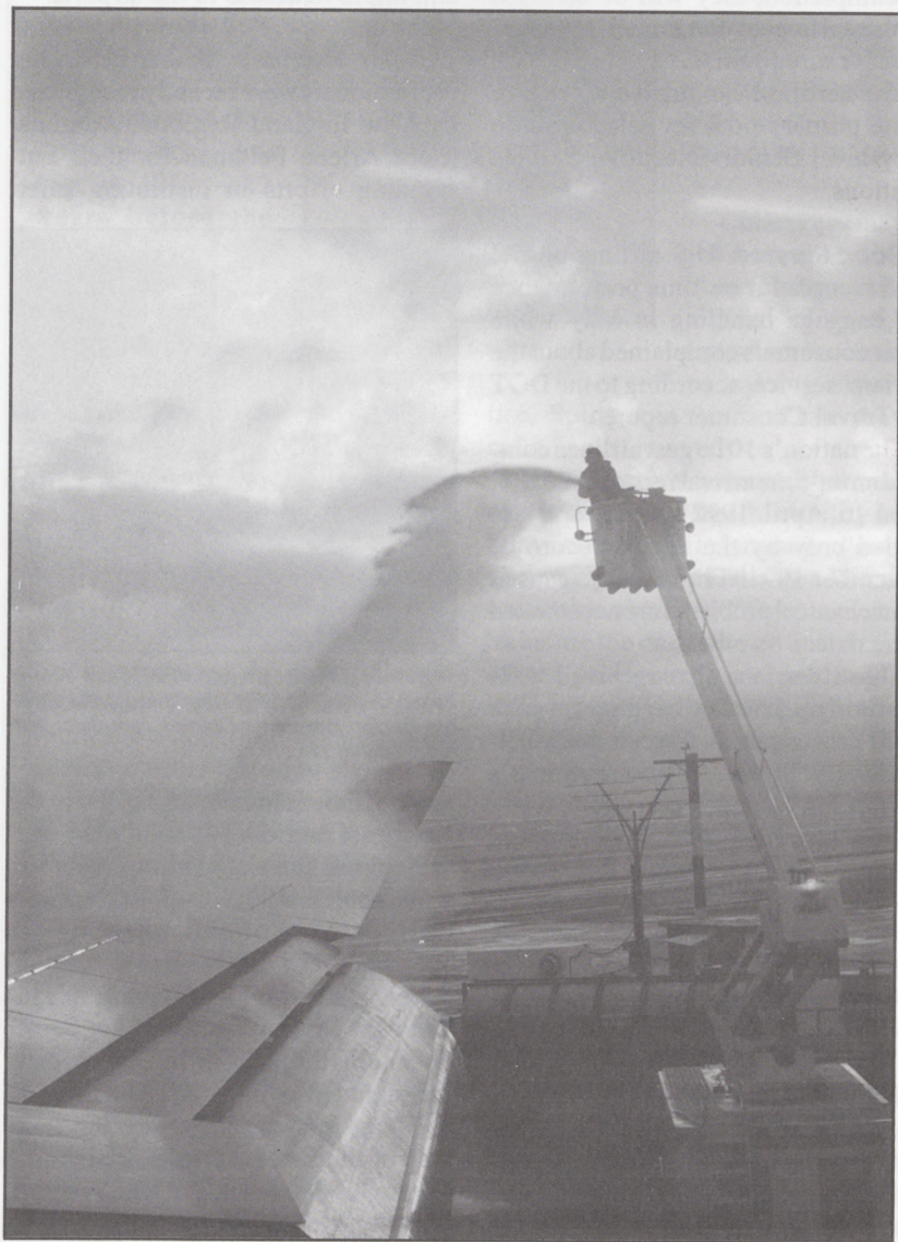
Airline worker sprays de-icing fluid on aircraft wing prior to a wintery takeoff.
