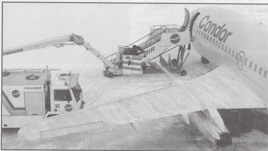
Airline worker prepares aircraft for a wintery takeoff by spraying wings with de-icing fluid.
