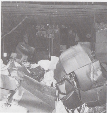
The remains of one of 39 fire tests on a "combi" aircraft.
