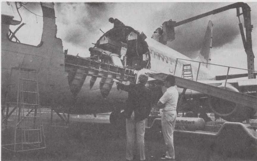
FAA's structural and corrosion actions stem from an April 1988 accident in which this Aloha Airlines 737 — with almost 90,000 flights — lost 18 feet off the top of its fuselage but managed to land safely. Although metal fatigue was the primary cause of the failure, corrosion was also found.
