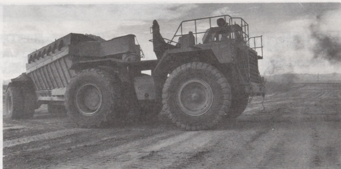
This huge tandem earth hauler is one of many clearing the site for the new Denver airport. It weighs more than 500,000 pounds when fully loaded.
