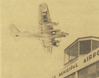
The first airliner with a pressurized cabin and four engines, a Boeing Stratoliner, flies over the Chicago Municipal Airport tower in 1940, wearing Transcontinental & Western Airlines colors. The airport is now known as Midway.
