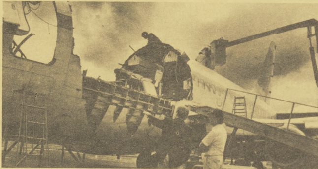
The April 1988 accident when an Aloha Airlines jet lost a chunk of its upper fuselage was a catalyst for sharpened attention to the aging aircraft issue.
