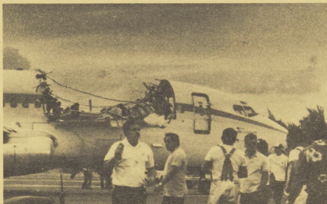
This Aloha Airlines 737 lost a big chunk of its fuselage last year.
