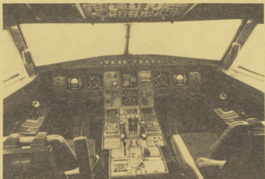
Cathode ray tube displays highlight A320's flight deck. Administrator Allan McArdor talks with Airbus official. He flew the airplane last summer. (top, left)
