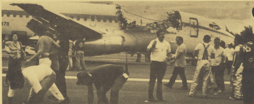
FAA called a special aging aircraft conference after this Aloha Airlines jet lost its top on April 28, 1988. Some 450 experts from across the country and 12 foreign nations attended.
