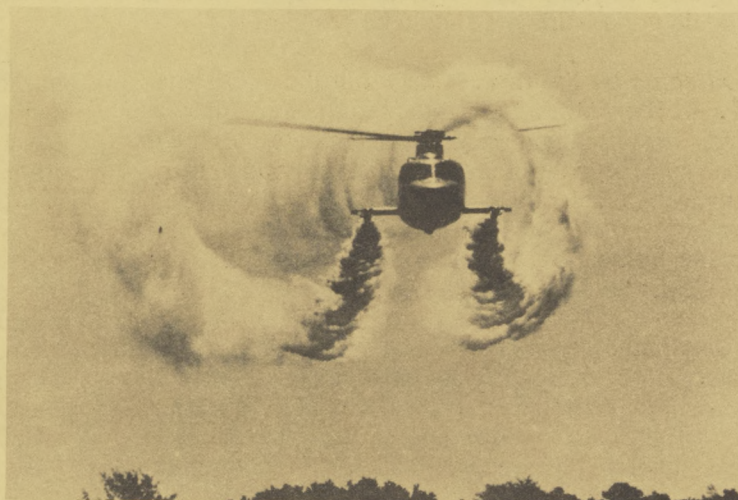
Smoke swirling from this helicopter makes air turbulence visible. It's part of ongoing testing at Atlantic City's Tech Center which is researching the wake vortex characteristics of commercial jet aircraft and helicopters and the impact of weather on turbulence.
