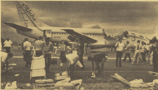
This photo, taken shortly after the Aloha jet landed on Maui, vividly shows the missing fuselage section.
