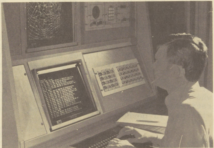
The specialist has text and graphic displays before him at the AFSS model 2 position console.
