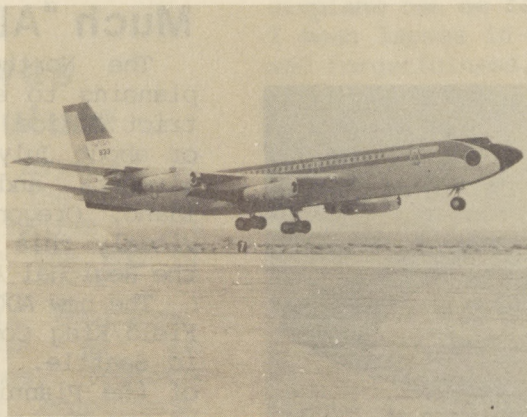
The Boeing 720 to be used in the controlled impact demonstration takes off on test flight from Edwards AFB. Engineering markings have since been added to help evaluate crash damage. (see page 2)
