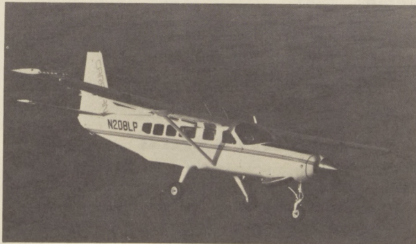
Cessna's Caravan I is a single-engine turboprop that can carry 14 passengers and cruises at 214 miles per hour.
