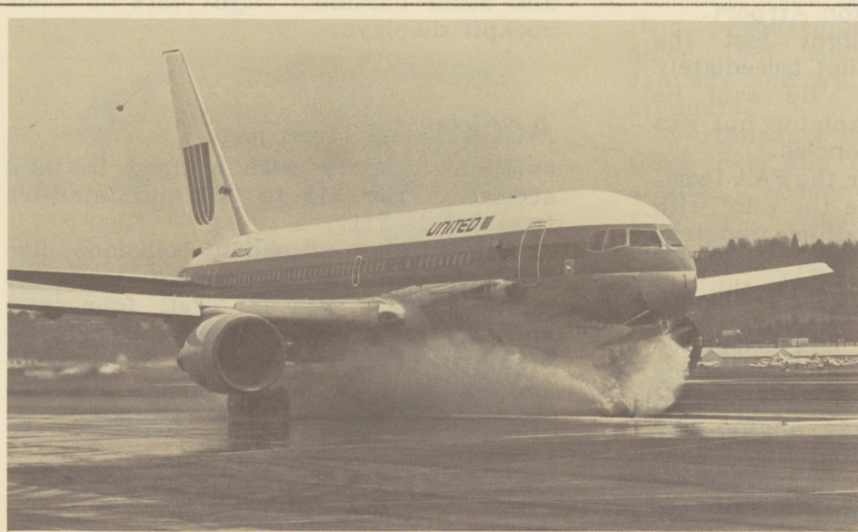
A United Airlines Boeing 767, like the one assisted to a safe landing by Denver ARTCC controllers, (See page 2) was used in the aircraft's FAA certification tests. Here the pattern of water thrown up by the nose wheel is checked.
