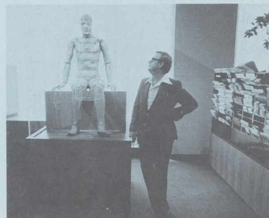
Anthropomorphic dummy (seated) is used in auto crash tests. At left, roadsign potpourri.
