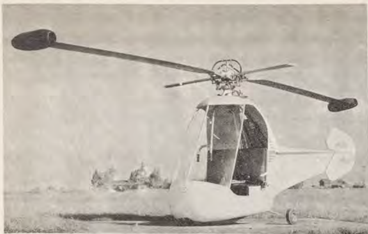
The Hiller "Hornet", a two-place ram-jet powered helicopter. (Photo courtesy Hiller Helicopters, Inc.)
