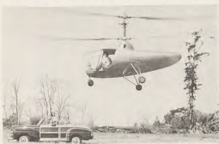
The Hiller "Commuter", one of the first successful co-axial rotor helicopters. (Photo courtesy Hiller Helicopters, Inc.)
