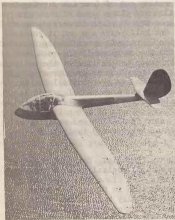
Pratt-Read glider with 55-foot wing span. This type holds the 2-place world altitude record.
