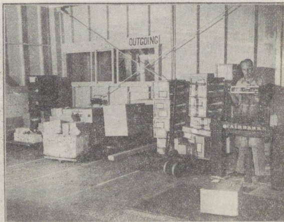
PACKAGES, CRATES, OR BOXES READY FOR SHIPMENT ARE ASSEMBLED AT THE FRONT OF THE WAREHOUSE NEAR THE MAIN SHIPPING-RECEIVING DOOR. SHIPMENTS ARE GROUPED BY TRANSPORTATION MEANS, I.E., PARCEL POST, EXPRESS, OR FREIGHT, THEREBY FACILITATING HANDLING AT THE END OF THE DAY, WHEN PICK-UP IS MADE. THE FLOOR SCALES ARE USED TO WEIGH LARGE ITEMS WHICH CANNOT BE HANDLED ON THE REGULAR SHIPPING LINE SCALE.
