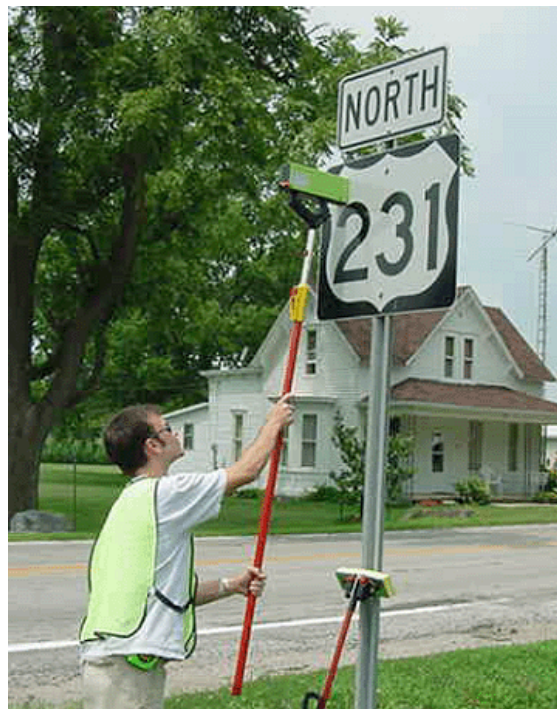
Figure 3-8: Picture of ART 920 with Extension Pole
