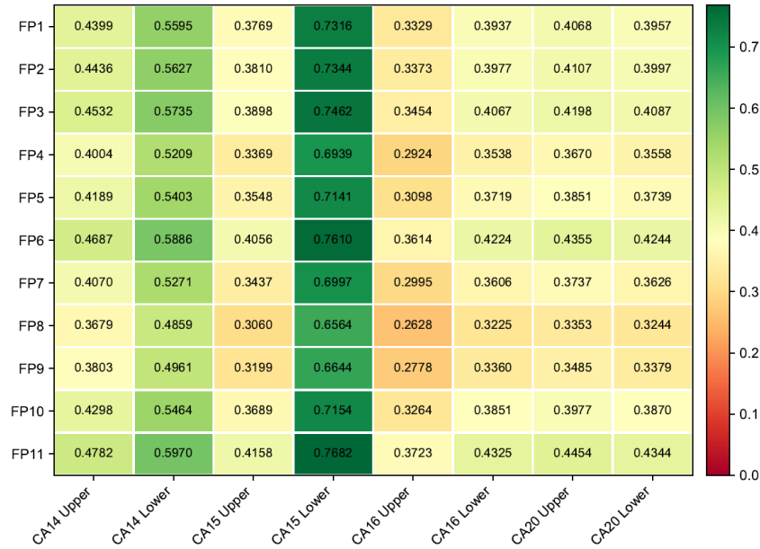
Figure 57. Graph. Predicted initial IFI ( a_{mix} + b_{mix} ) for all chip seal aggregate-gradation combinations.
