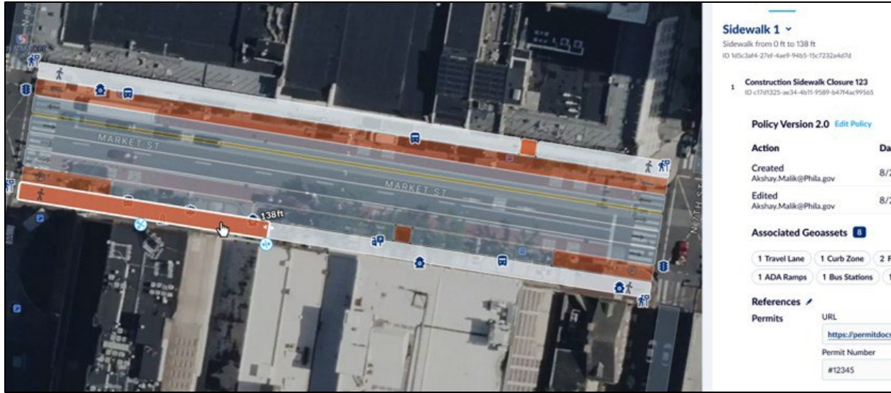
Figure 6. Road Rules Demonstration: Lane-level mapping and editing; Tagging of impacted Geo-assets. Source: INRIX
