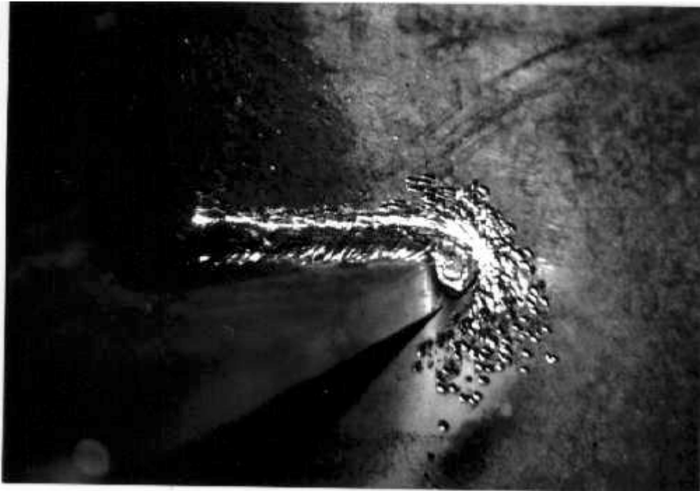
Figure 4.10 Photograph of the peened bottom flange weld area
