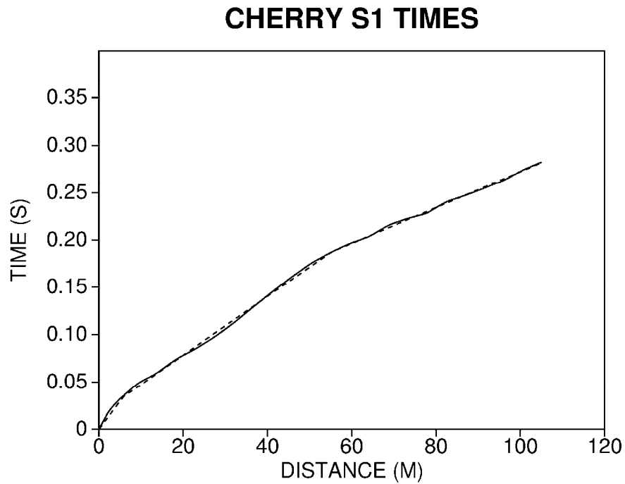
Figure 2-12 Travel-time curve from picked S-arrivals of refraction record section
