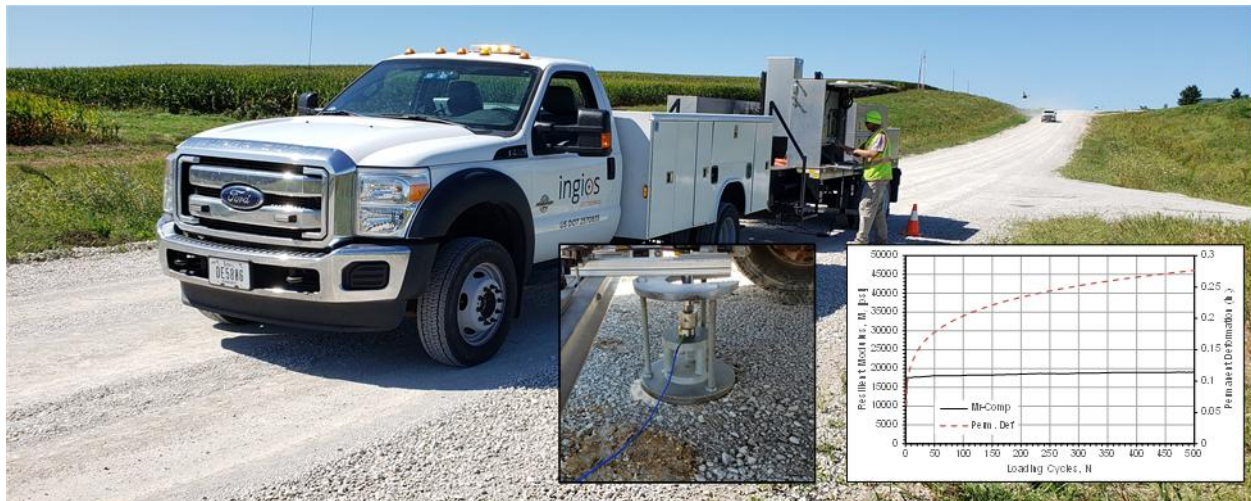
Figure 7. Cyclic APLTs to determine in situ composite resilient modulus ( M_r ) and permanent deformation ( p ) or rutting
