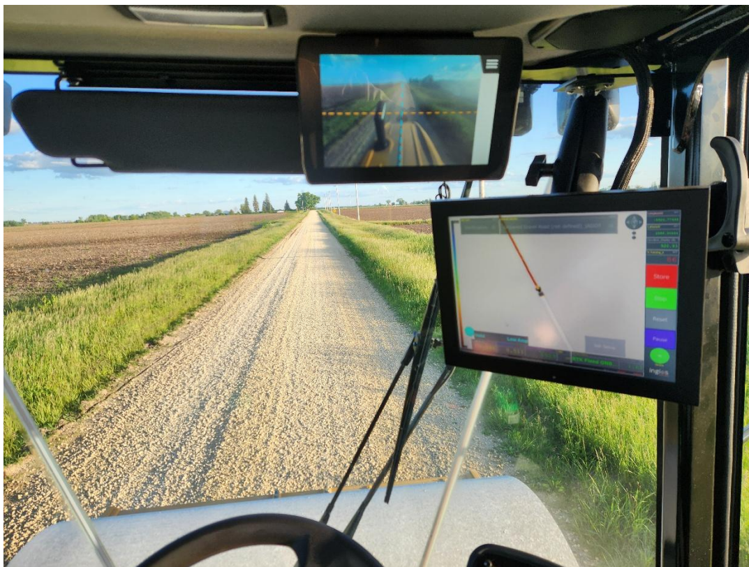
Figure 9. COMP-Score RT enabled roller performing modulus mapping on an unpaved gravel road
