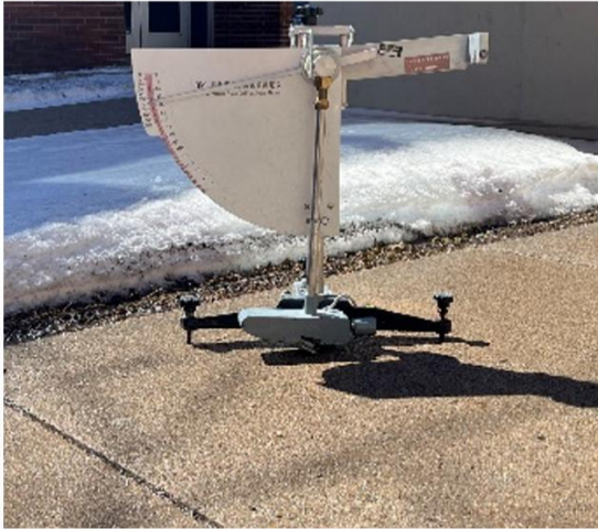
Figure 3-4: British Pendulum Tester for Measuring Skid Resistance of Pavement Surface.
