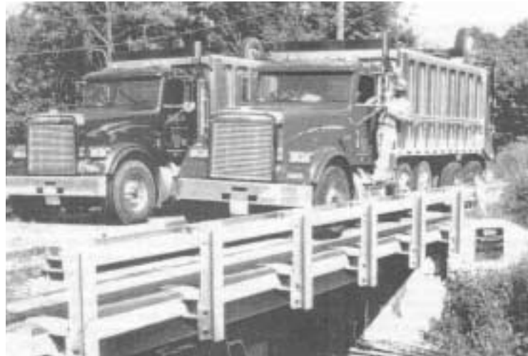
Figure 3.15. Live load test of the “Tech 21” bridge (Foster et al. 2000)
