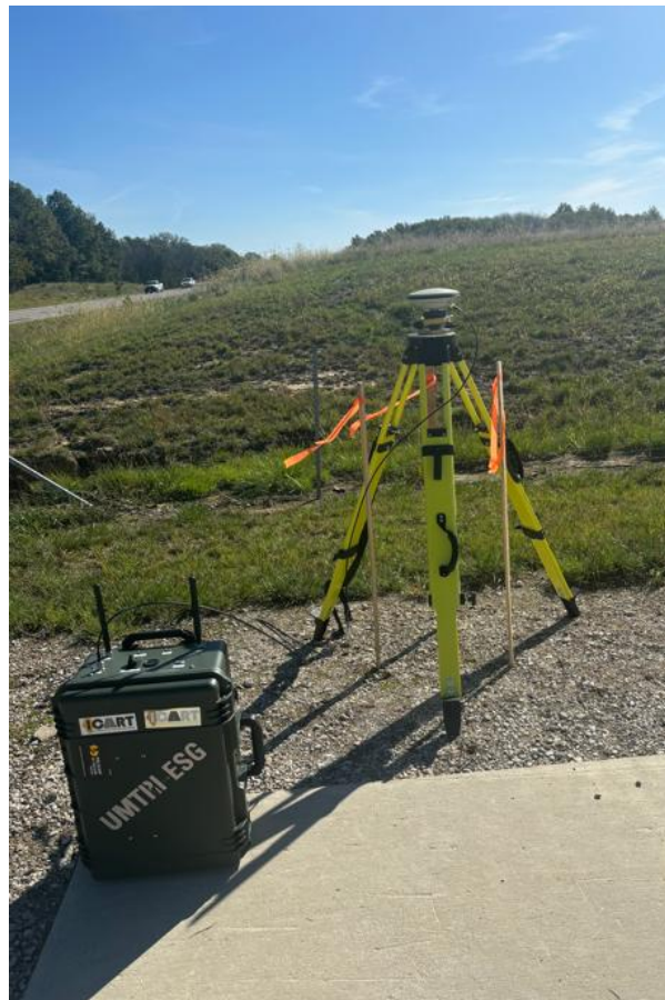
Figure 11. Mobile GPS base station.
