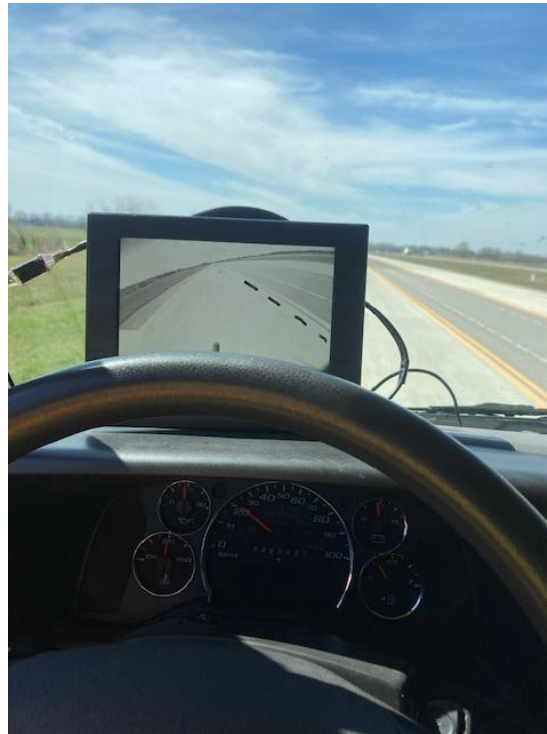
Figure 12. Dashboard monitor for lane tracking feedback.
