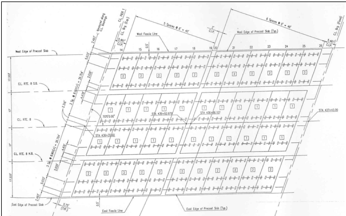
Fig. 30. Typical precast slab layout plan for one bridge in Seymour, CT (CT-DOT, 1992)
