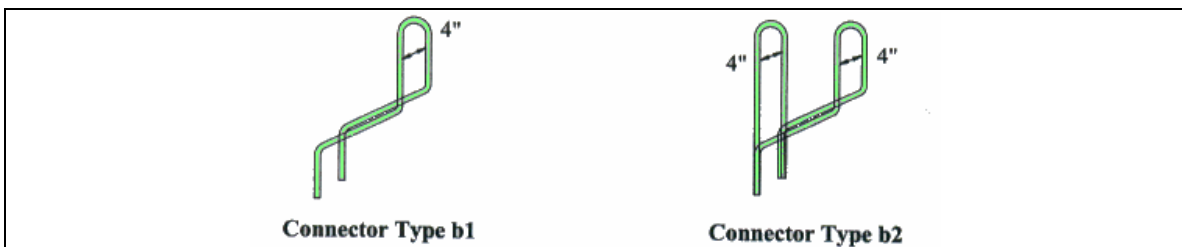
Fig. 19. Connectors for debonded system (Tadros and Baishya, 1998)
