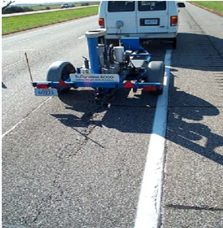
Figure 13: FWD testing on Site 1 (I-65 North of Lafayette).
