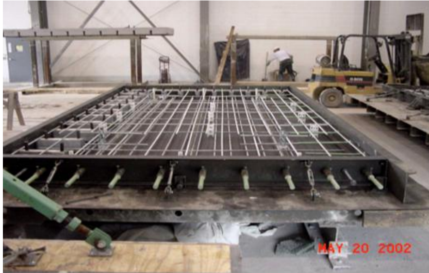
Figure 5.2 Precast Concrete Slab Form (18)
