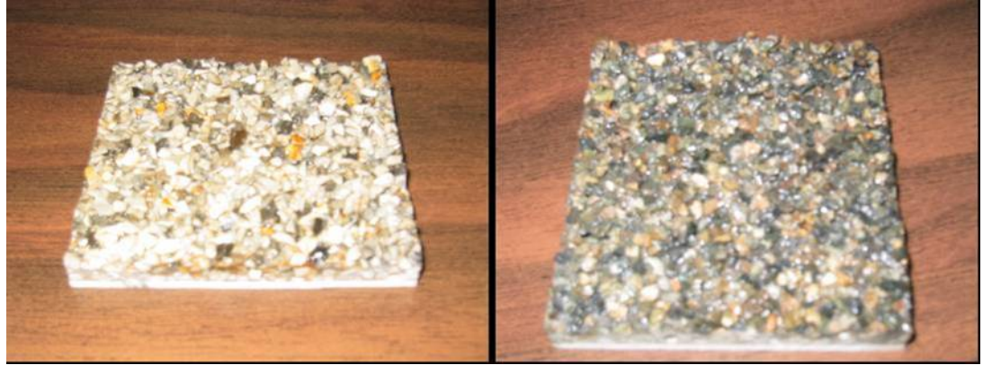
Figure 4- 11 Sample of wearing surface used in Sintz Road over Rock Run Bridge
