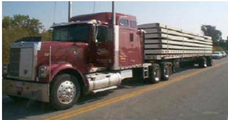
Figure 5-4 Panels Transported to Job Site (Source: Busel and Lockwood 2000)
