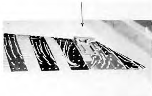
Figure 7. Surface flow visualization on wing upper surface with spoiler and delta tip.
