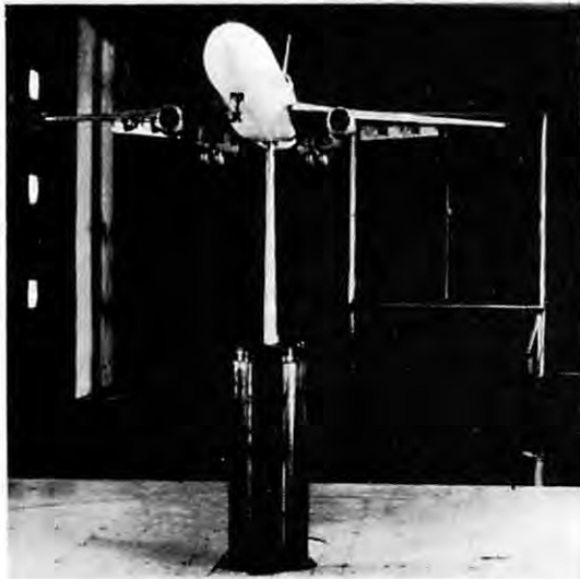
Figure 25. Photograph of the DC-10-30 airplane model and traverse mechanism in the Langley V/STOL tunnel.
