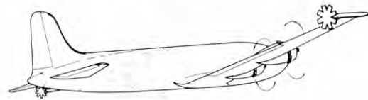
Figure 2. C-54G aircraft with splines installed.
