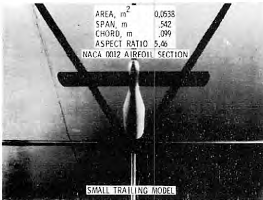
Figure 28. Photograph of unswept trailing wing model on traverse mechanism. (Sensor models used for L-1011 airplane model tests.)
