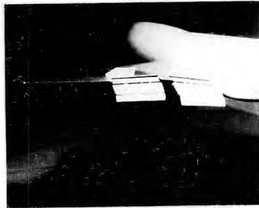
Figure 14. Photograph of flight spoiler segments 1 and 2 simulated with wedges on B-747 airplane model. Spoiler deflected 45°.
