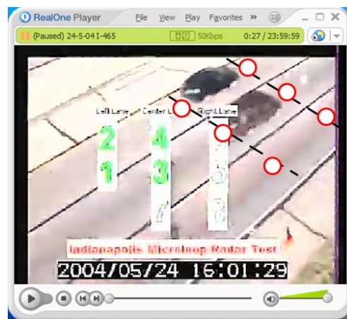
Figure 4-5: Screen capture of the video overlay of detector status with approximate location of microloops shown (Channels 1, 2, 3 and 4 are ON)
