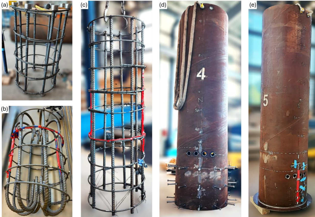
Figure 3-4 Rebar Cages—(a) Headed, (b) Hooked, and (c) Straight; and Welded Specimen Connections—(d) Stud and (e) Ring
