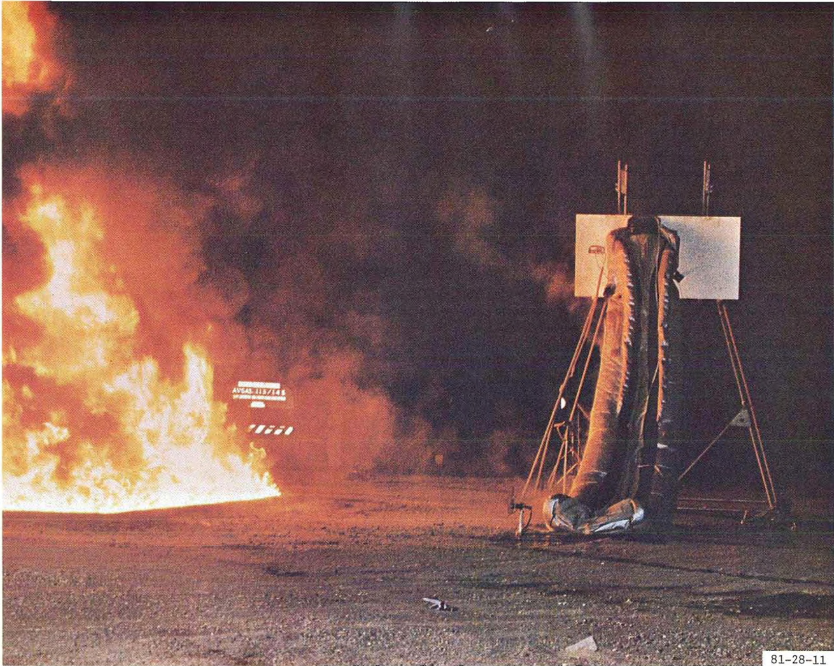
FIGURE 12. ALUMINIZED URETHANE NYLON SLIDE FAILURE DURING TEST; TEST 16B
