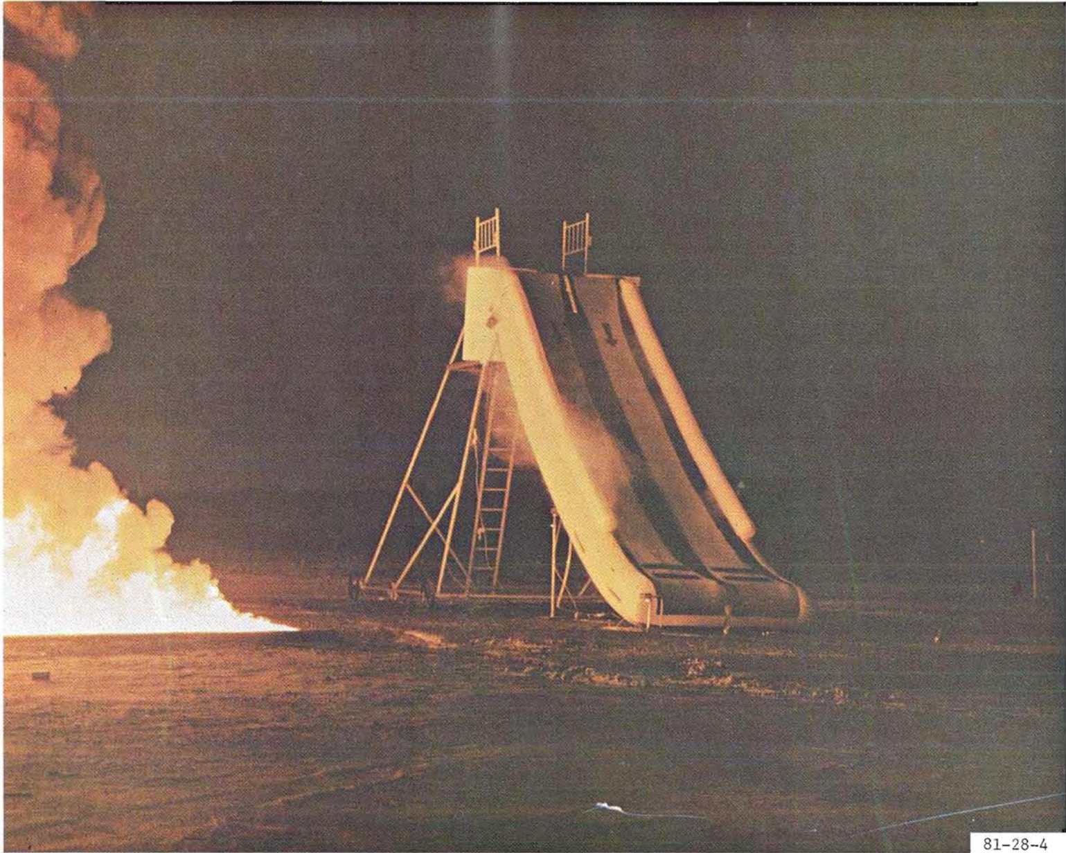
FIGURE 5. URETHANE NYLON SLIDE SMOKING DURING TEST; TEST 3B
