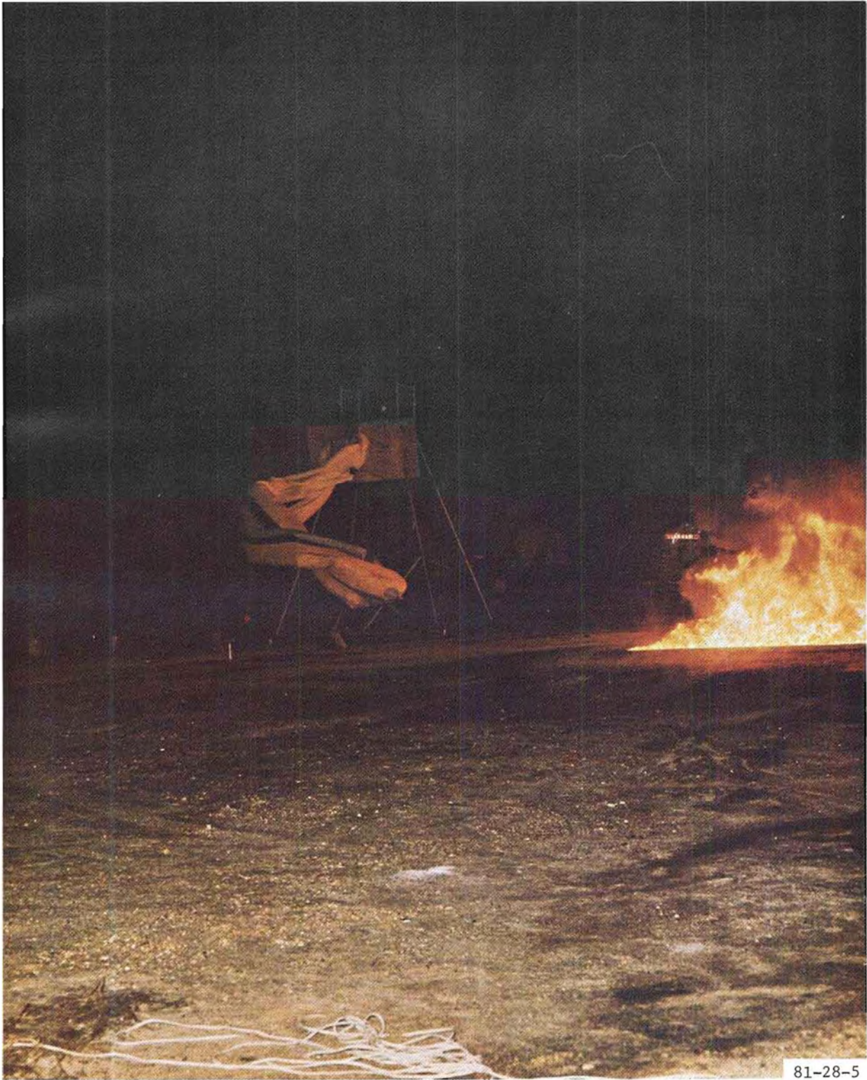
FIGURE 6. CATASTROPHIC FAILURE OF URETHANE NYLON SLIDE; TEST 8A
