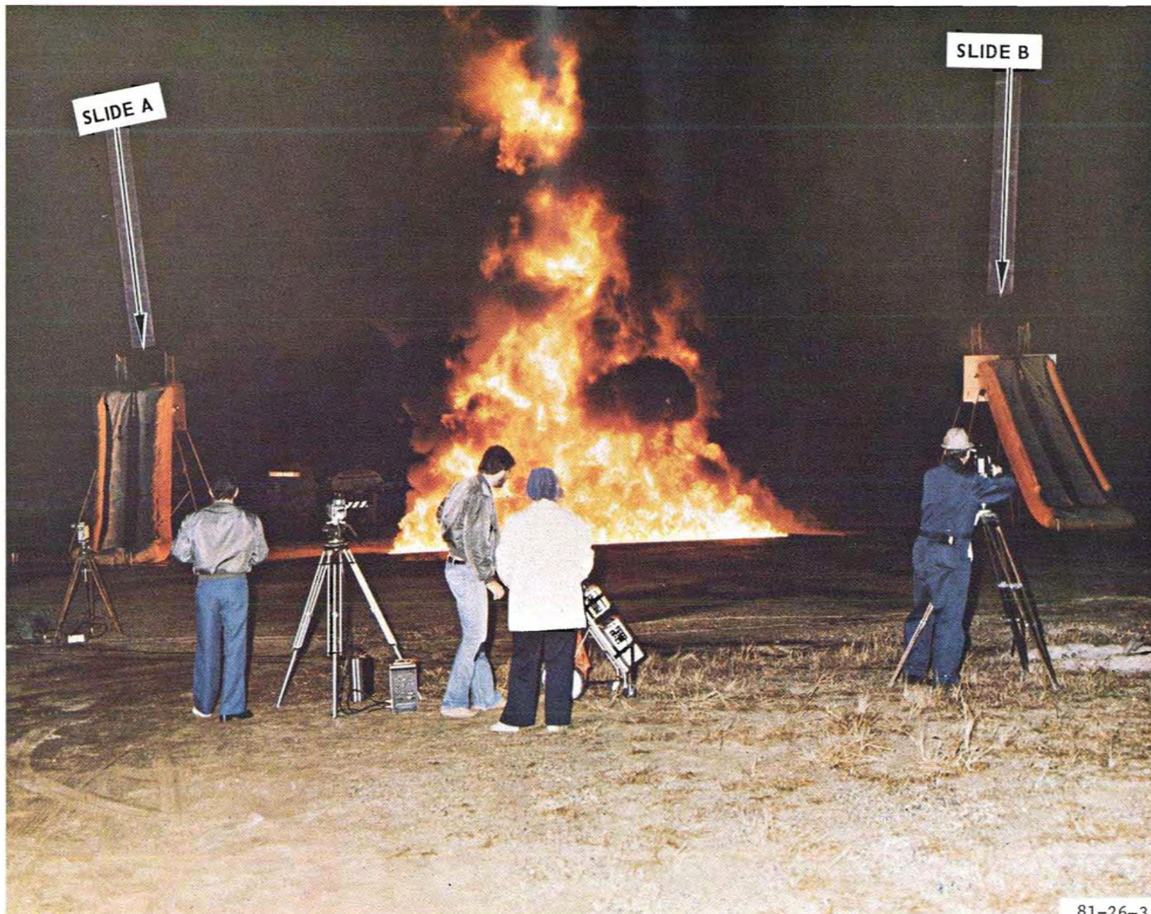
FIGURE 4. FULL-SCALE FIRE TEST SET-UP; TEST 5
