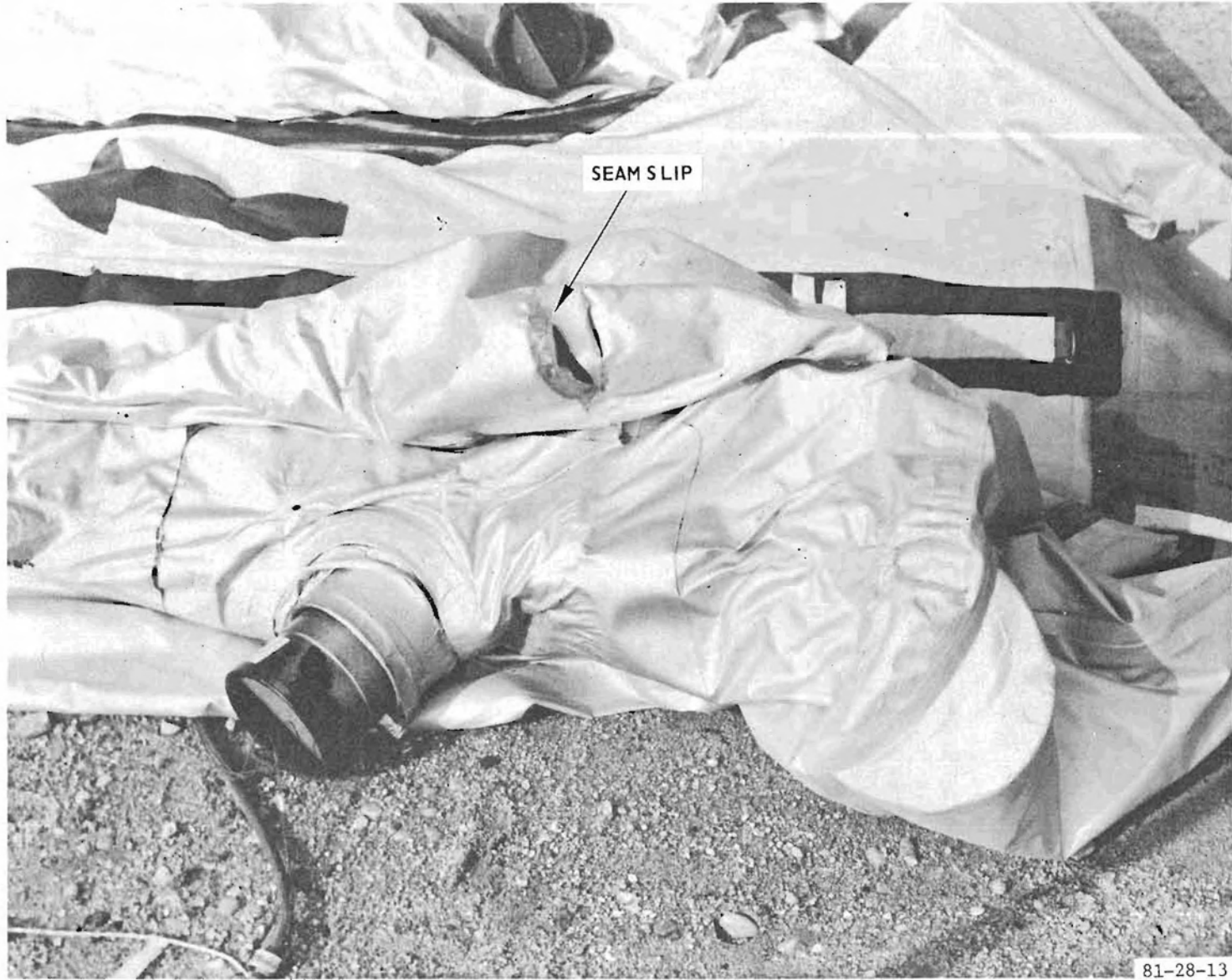
FIGURE 14. ALUMINIZED URETHANE NYLON SEAM SLIPPAGE; TEST 19
