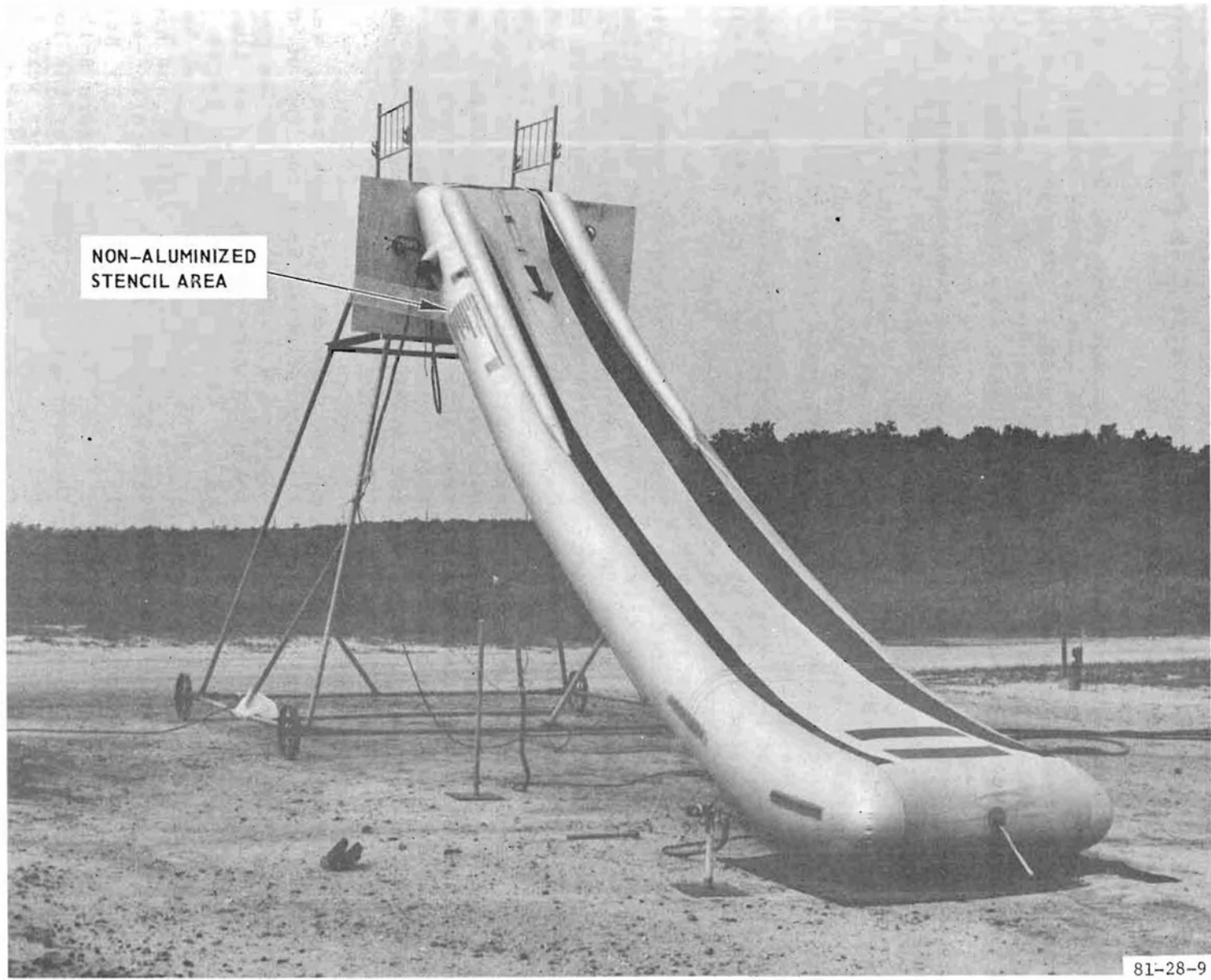
FIGURE 10. ALUMINIZED URETHANE NYLON WITH STENCILING SHOWING; TEST 16B
