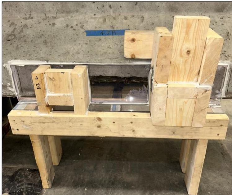
Figure 61. Photo. Formwork with one chimney for repair 4.2RBZ.
