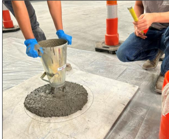
Figure 43. Photo. Inverse slump cone test for the SCC mix.
