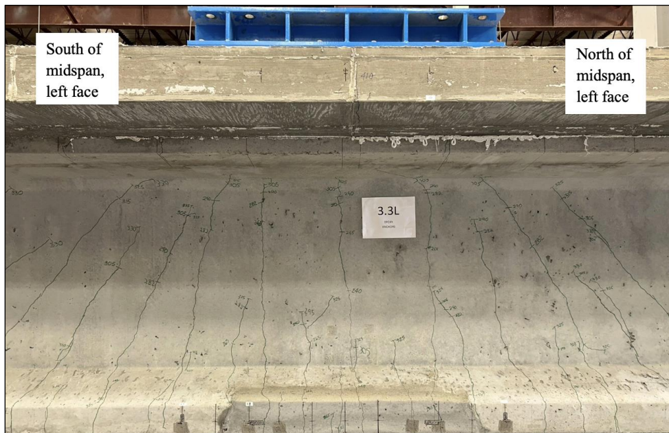
Figure 159. Photo. Test 3.3.F (repair 3.3RBF, 3.3LBF) overall crack pattern at the final load of 330 kip. Extensive flexural cracks occurred in the bottom flange repair (left face of girder pictured).
