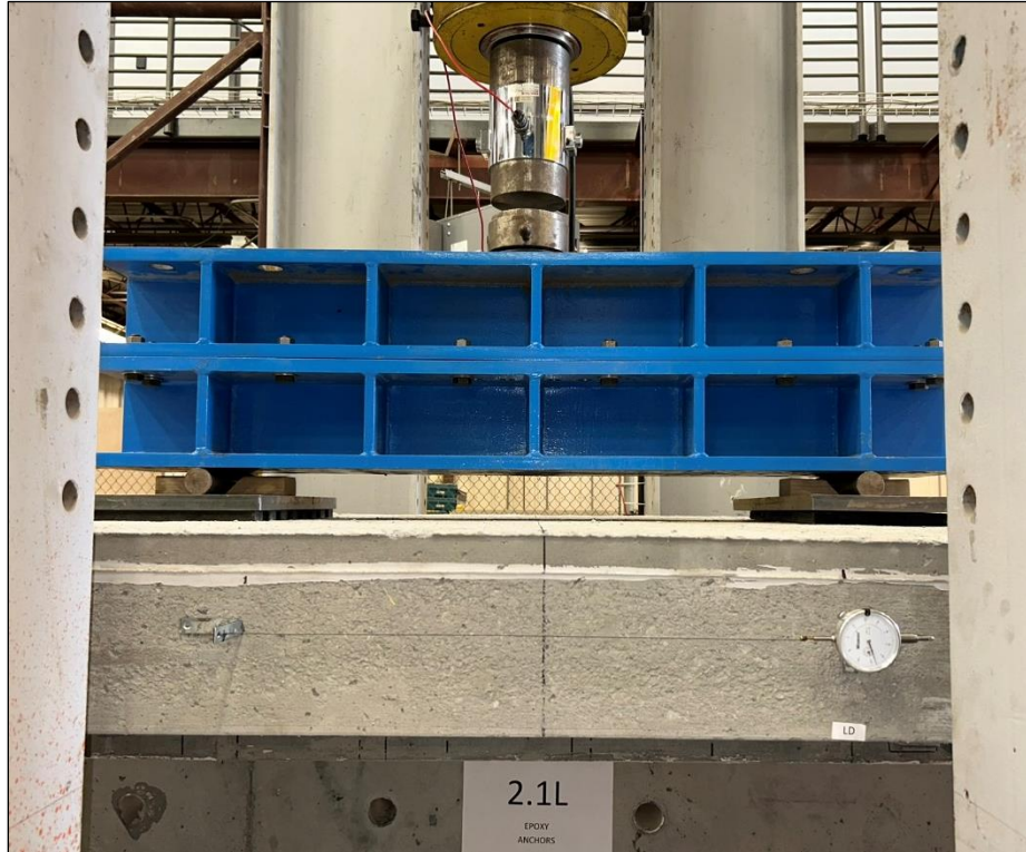
Figure 108. Photo. Test 2.1.S (repair 2.1RTF, 2.1LTF) spreader beam with two rollers spaced 4 ft apart and 51 in. long.
