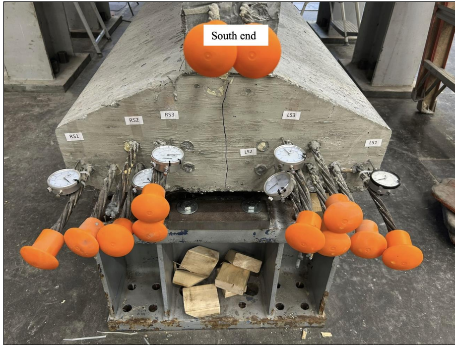
Figure 119. Photo. Test 2.2.S (repair 2.2LTF) south end cross-section crack at 281 kip.
