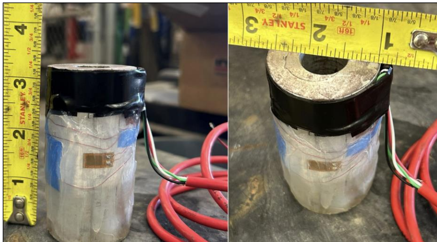
Figure 71. Photo. Load cells.
