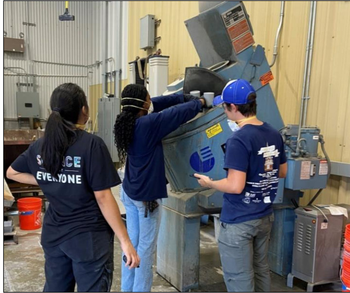
Figure 21. Photo. Concrete mixing 2-ft 3 batches with Eirich mixer.
