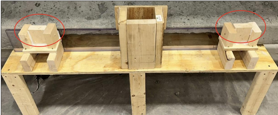
Figure 8. Chimney formwork example.
