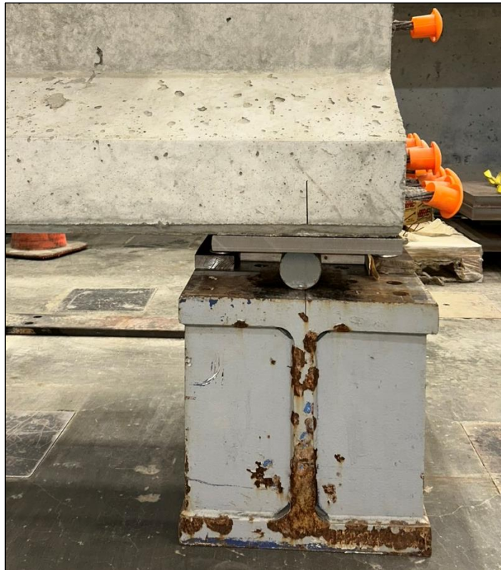
Figure 79. Photo. Girder boundary conditions.
