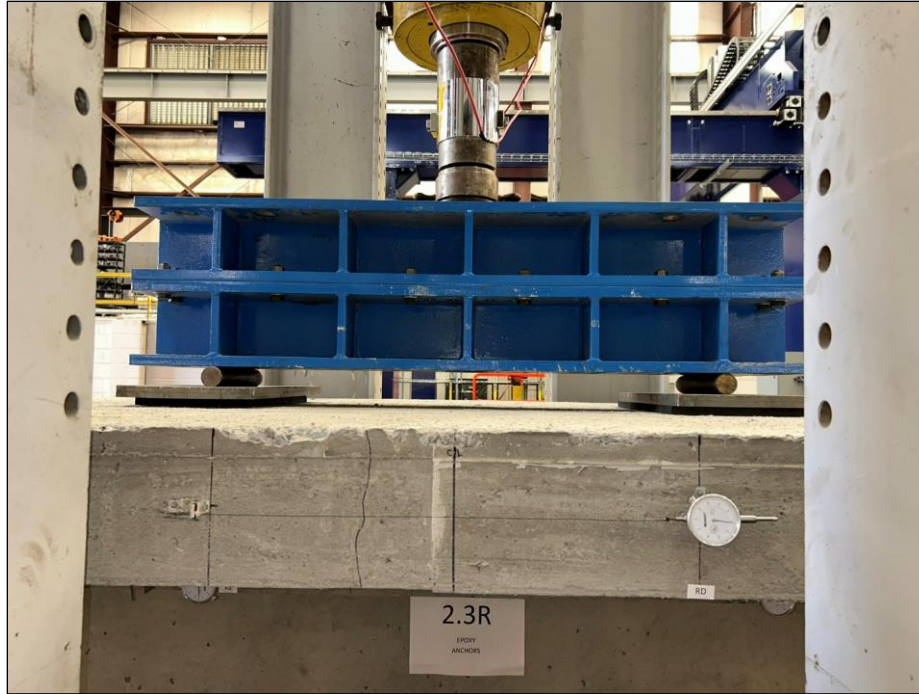
Figure 126. Photo. Test 2.3.F (repair 2.3LTF) spreader beam four-point bending configuration near midspan, simulating a two-axle truck load to create maximum tensile stress in the top flange.
