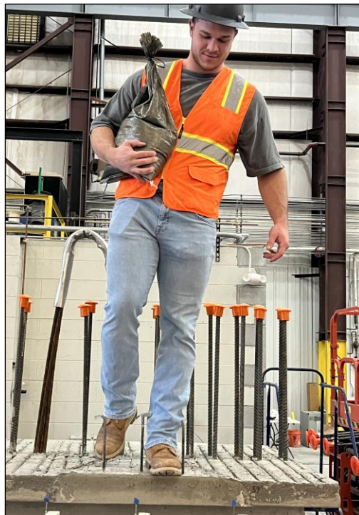
Figure 26. Photo. Point load of 250 lb on the top flange.
