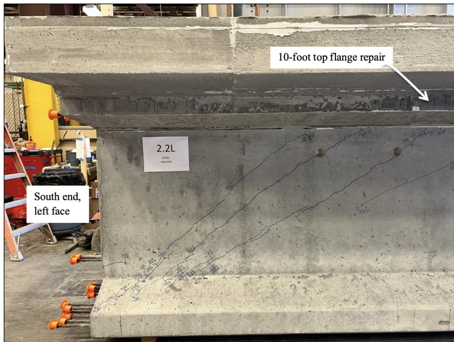
Figure 122. Photo. Test 2.2.S (repair 2.2LTF) final shear cracks on repaired face at 424 kip. The longest top flange repair length is 126 in. (left face of girder pictured).
