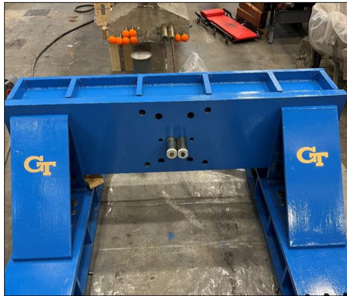
Figure 69. Photo. Dead end abutment anchored to the strong floor.
