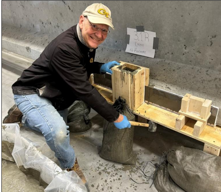
Figure 51. Photo. Vibrating the formwork with a rubber mallet.
