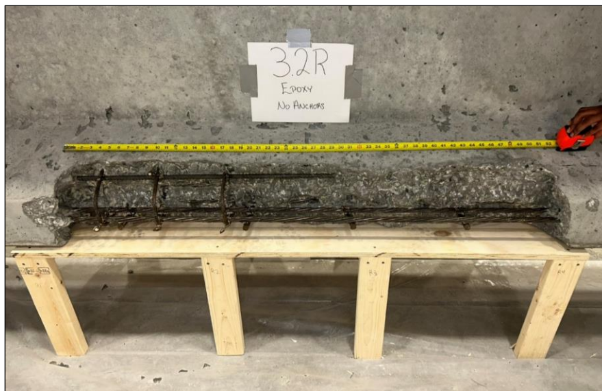
Figure 48. Photo. Bottom flange repair 3.2RBF with no post-installed anchors.
