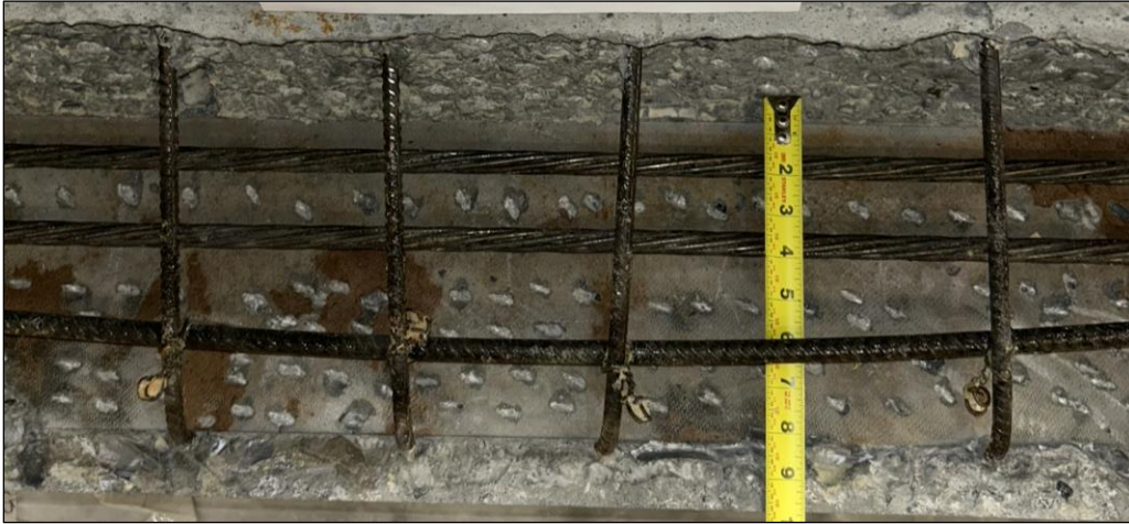
Figure 15. Photo. Roughened 0.25-in. amplitude surface.
