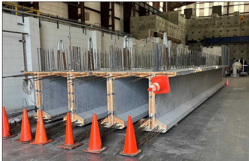
Figure 11. Photo. BT-54 girders in the Georgia Tech SEML.
