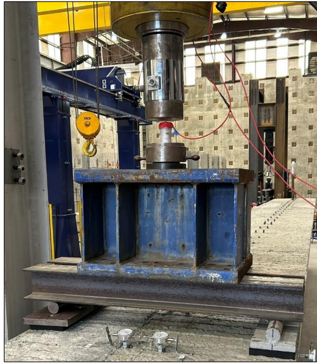
Figure 80. Photo. Top flange test setup.
