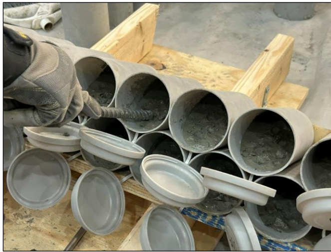
Figure 75. Photo. Roughening the surfaces of the bottom half slant shear cylinders, which were cast at a 30-degree angle.
