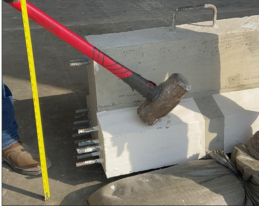
Figure 40. Photo. Strength and efficacy test of 12-gauge wire reinforcement and concrete anchors by striking with a 16-lb sledgehammer.
