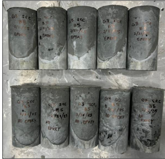
Figure 77. Photo. Demolded slant shear cylinders.
