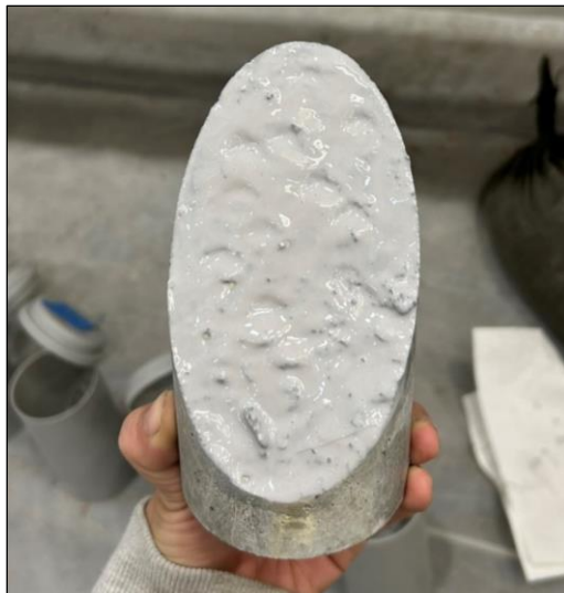
Figure 76. Photo. Sikadur-32 coat on angled surface of slant shear cylinders.
