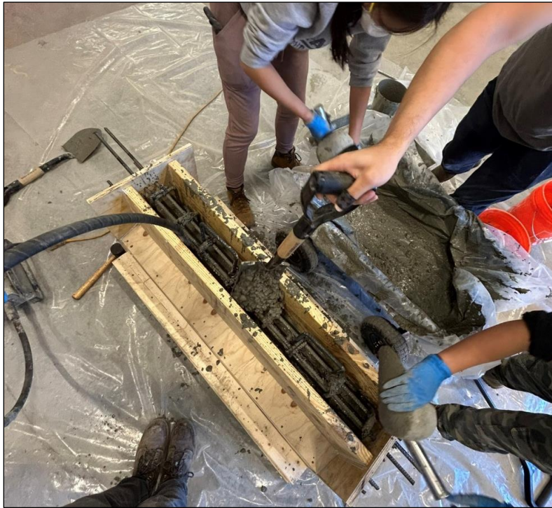
Figure 30. Photo. Mini girder construction using the same concrete mix as used in the full-size BT-54 girders.
