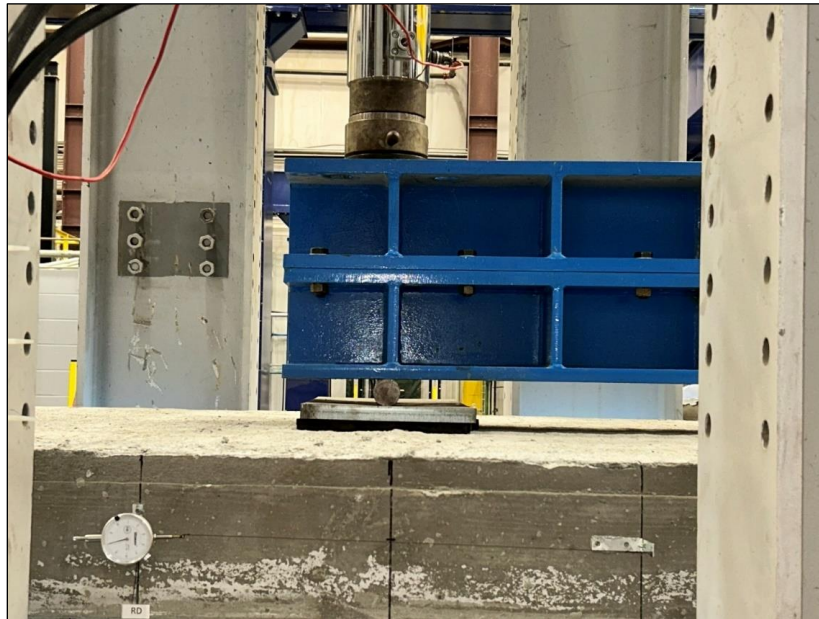
Figure 134. Photo. Test 3.1.S (repair 3.1RBF, 3.1LBF) spreader beam configuration with the hydraulic ram located directly above the load point closest to the north girder bearing.
