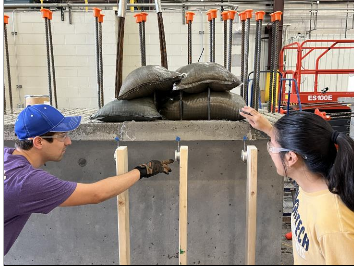
Figure 27. Photo. Distributed load of 50 psf on the top flange.
