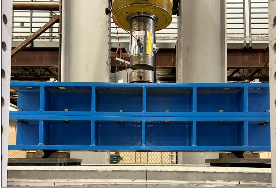
Figure 78. Photo. General spreader girder configuration.
