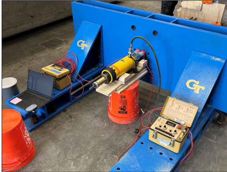
Figure 72. Photo. Live end configuration with load cells and a center hole jack.
