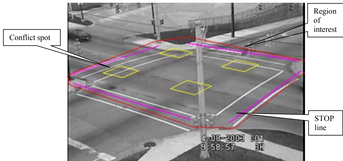
Figure H-1: Conflict spots, STOP lines and Region of Interest on the Screen Capture of the Intersection 97901 (SR-26 @ 18 th St)
